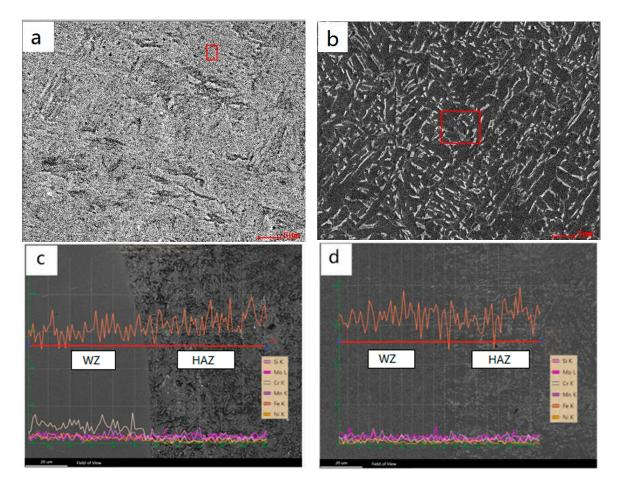
**Figure 6.** EDS analysis of the welds: (**a**) welding seam of LTT ;(**b**) welding seam of ER110S-G; (**c**) the line scanning of LTT ;(**d**) the line scanning of ER110S-G.
