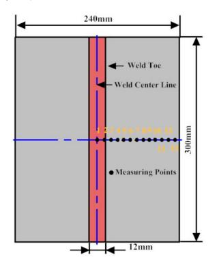
Figure 11. The measuring points of residual stress.
