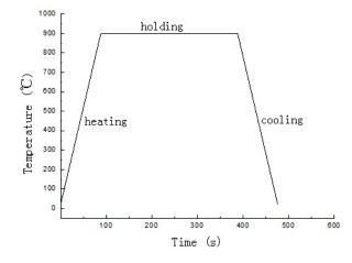
Figure 9. The schematic of thermal simulation cycling curve.
