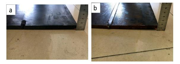
Figure 13. Welding deformation of (a) LTT and (b) ER110S-G weld joints.
