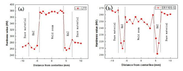
Figure 7. Micro-hardness of weld joints (a) LTT joint and (b) ER110S-G joint.
