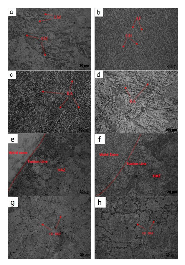
**Figure 4.** Microstructure of welded joints :(**a**) welding seam of LTT; (**b**) welding seam of ER110S-G; (**c**) the third layer of LTT; (**d**) the first layer of LTT; (**e**) fusion zone of LTT; (**f**) fusion zone of ER110S-G; (**g**) Coarse grain zone of LTT; (**h**) Coarse grain zone of ER110S-G.
