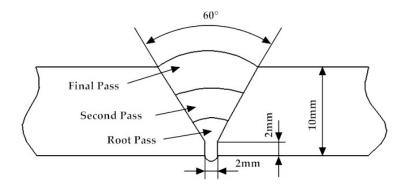
Figure 3. Joint groove.
