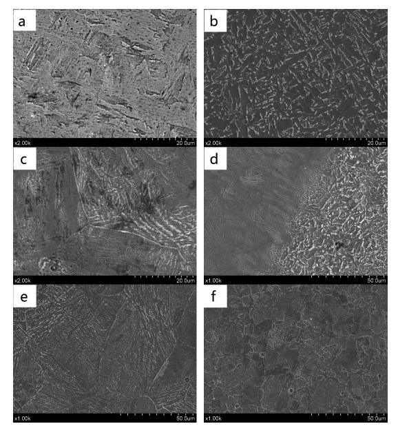
**Figure 5.** SEM morphology of welded joints :(**a**) welding seam of LTT; (**b**) welding seam of ER110S-G (**c**) retained austenite (RA) of LTT; (**d**) fusion zone of LTT; (**e**) Coarse grain zone of ER110S-G; (**f**) fine grain zone of ER110S-G.
