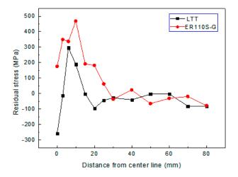
Figure 12. The residual stresses distribution of weld joints.
