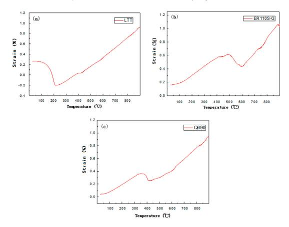
Figure 10. Strain curves with temperature of different weld metals (a) LTT weld, (b) ER110S-G weld, and (c) base metal Q690.
