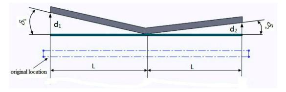
Figure 14. Angular distortion calculation model.
