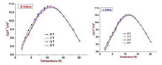
**Figure 5.** Temperature dependence of the heat capacities  $C_p/T^3$  of D-, L-valine. Crystals as a function of external magnetic field with H//b axis.
