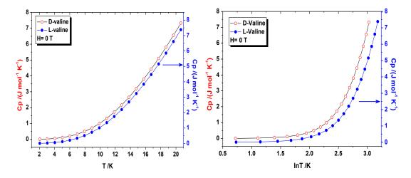
**Figure 3.** Low temperature  $C_p$  versus *T* and  $C_p$  versus  $\ln T$  of D- and L-valine at zero-field.
