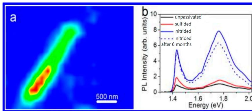
**Figure 11.** (a)  $\mu$ -PL intensity distribution over the surface of nitrided n-GaAs NW; (b)  $\mu$ -PL spectra taken from the middle section of the nitrided, sulfided, and unpassivated NWs. A  $\mu$ -PL spectrum from a nitrided NW measured after six months of storage in ambient air is also presented. Reproduced with permission from [48], copyright American Chemical Society (2015).
