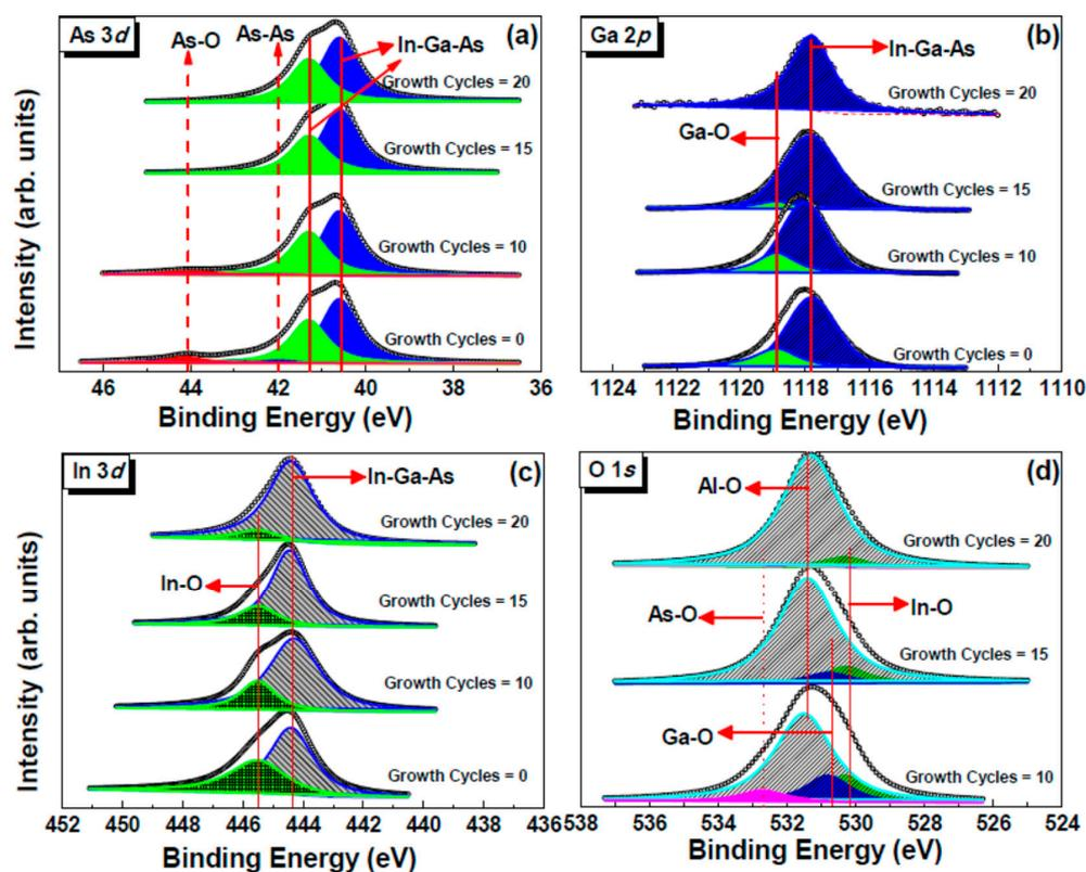
**Figure 4.** XPS spectra of As 3d (a), Ga 2p (b), In 3d (c) and O 1s (d) with the influence of ALD- $\text{Al}_2\text{O}_3$  growth cycles. Reproduced with permission from [31], copyright American Chemical Society (2016).
