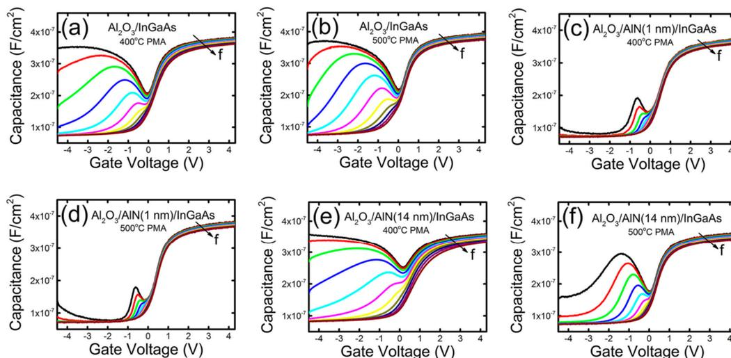
**Figure 12.** Typical capacitance-voltage characteristics at 400 Hz–1 MHz frequency range of (a,b) Au/Cr/ $\text{Al}_2\text{O}_3$  (18 nm)/InGaAs; (c,d) Au/Cr/ $\text{Al}_2\text{O}_3$  (17 nm)/AlN (1 nm)/InGaAs and (e,f) Au/Cr/ $\text{Al}_2\text{O}_3$  (4 nm)/AlN (14 nm)/InGaAs gate stacks measured after annealing at 400 °C (a,c,e) and at 500 °C (b,d,e) in  $\text{N}_2$  for 5 min. Reproduced with permission from [49], copyright AIP (2017).
