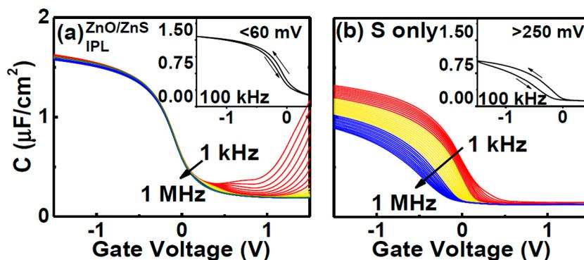
**Figure 8.** C-V characteristics of  $(\text{NH}_4)_2\text{S}$  cleaned  $\text{HfO}_2$ /p-InGaAs MOSCAP with (a) and without (b) ZnO/ZnS IPL. Reproduced with permission from [37], copyright The Japan Society of Applied Physics (2016).
