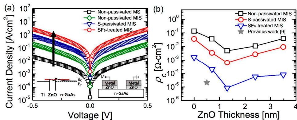
**Figure 10.** (a) I-V characteristics and (b) specific contact resistivity for metal semiconductor (MS) contact and MIS contacts. The ZnO is used as interlayer and 1.3 nm ZnO is considered the optimal thickness in both MIS contacts. Insets in (a) show a band diagram of the MIS contact (left) and a schematic of the electrical measurements of the MIS contact (right). Reproduced with permission from [47], copyright IEEE (2016).
