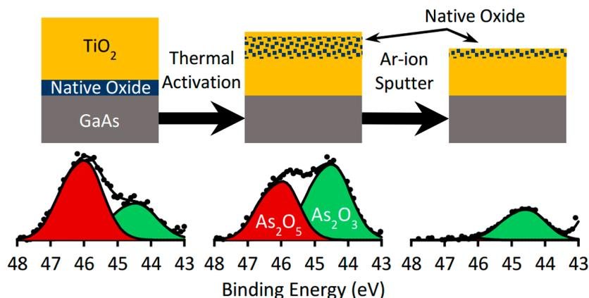
**Figure 9.** Schematic illustrating the experimental steps used to decouple the native oxide transport and removal processes. Reproduced with permission from [38], copyright American Chemical Society (2016).
