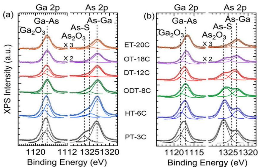
**Figure 2.** The Ga-2p and As-2p X-ray photoelectron spectroscopy (XPS) spectra for GaAs passivated by six alkanethiols after (a) 3 min and (b) 30 min of ambient exposure. Reproduced with permission from [21], copyright Elsevier B. V. (2016).
