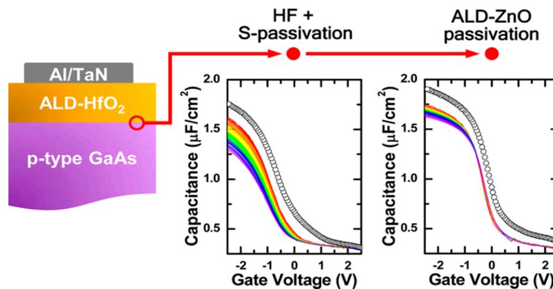
**Figure 7.** The C-V characteristics of HF+ (NH<sub>4</sub>)<sub>2</sub>S cleaned HfO<sub>2</sub>/p-GaAs MOSCAP with and without 10 cycle ALD–ZnO passivation layer. Reproduced with permission from [34], copyright American Chemical Society (2014).
