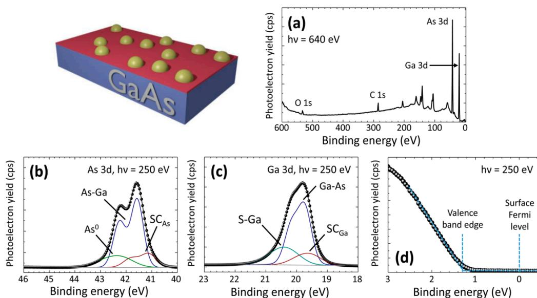
**Figure 1.** GaAs surface after thermal desorption of the sacrificial SAM. (a) The overview SRPES spectrum indicates low O and C surface contamination. The (b) As 3d and (c) Ga 3d spectra also demonstrate the absence of surface oxides above the detection limit. (d) The valence band spectrum indicates the absence of strong band bending near the surface. Reproduced with permission from [20], copyright American Chemical Society (2016).
