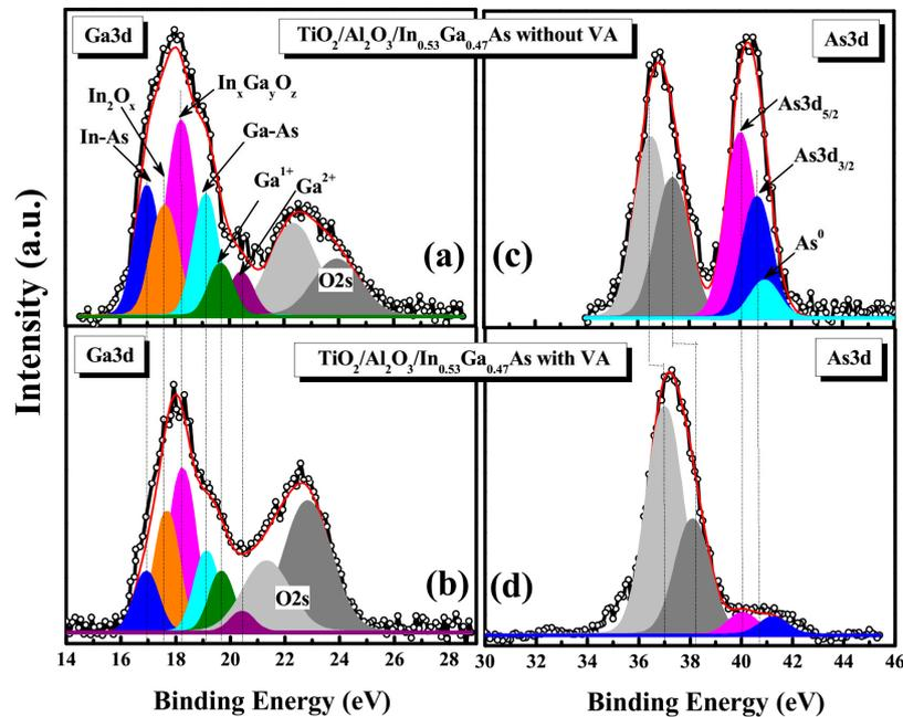
**Figure 5.** XPS spectra of Ga 3d (a,b) and As 3d (c,d) from TiO<sub>2</sub>/Al<sub>2</sub>O<sub>3</sub>/In<sub>0.53</sub>Ga<sub>0.47</sub>As structure without and with vacuum annealing (VA). Reproduced with permission from [8], copyright American Chemical Society (2016).
