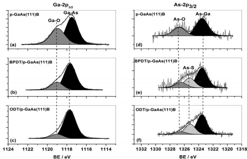
**Figure 3.** XPS spectra of Ga-2p and As-2p for p-GaAs substrate exposed to ambient after etching (a,d), BPDT passivation (b,e) and ODT passivation (c,f). Reproduced with permission from [22], copyright Elsevier B. V. (2016).
