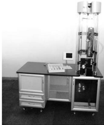
**Figure 3.** Machine for preparation of cast glass-coated amorphous micro- and nanowires (CGCFMWs) by the Taylor–Ulitovsky method.
