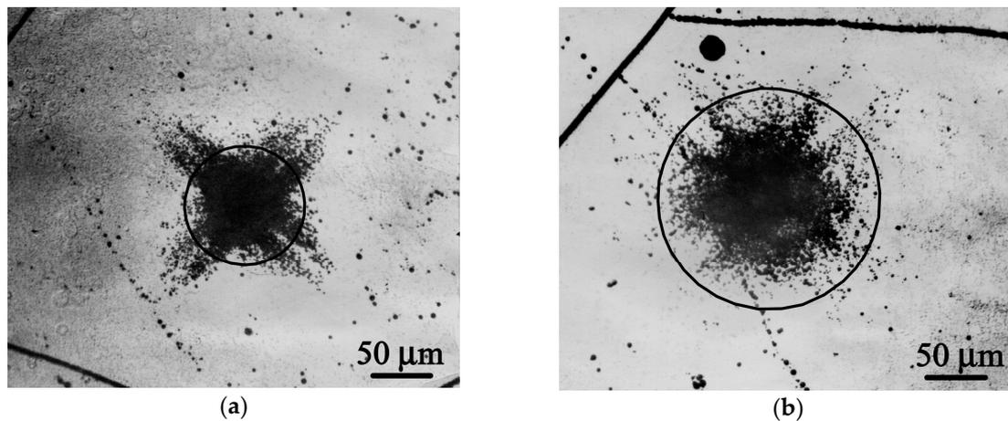
**Figure 5.** Dislocations around indentation print for single crystal Mo (001), revealed by etch pits method. The circles with radius  $b_S$  are plotted on dislocation rosettes: (a)  $t = 20\text{ }^{\circ}\text{C}$ ,  $HM = 1.998\text{ GPa}$ ,  $b_S = 47.7\text{ }\mu\text{m}$  [34]; (b)  $t = 300\text{ }^{\circ}\text{C}$ ,  $HM = 1.026\text{ GPa}$ ,  $b_S = 87.2\text{ }\mu\text{m}$ , present work.
