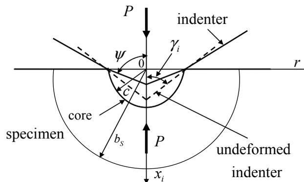
**Figure 1.** Scheme of interaction of an indenter and a specimen under a load  $P$  in a spherical coordinate system  $Or\theta\psi$ ,  $HM = P/(\pi c^2)$ .
