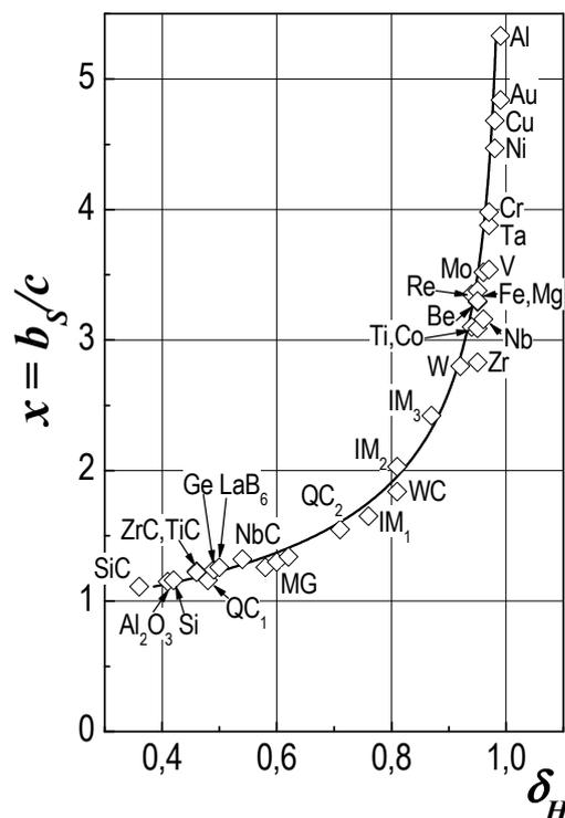
**Figure 2.** Relation between the plasticity characteristic  $\delta_H$  and the relative size of the elastoplastic deformation zone  $x$ . Curve was constructed on the basis of Equation (12) for  $z = 0.38$  and  $\nu_S = 0.27$ .
