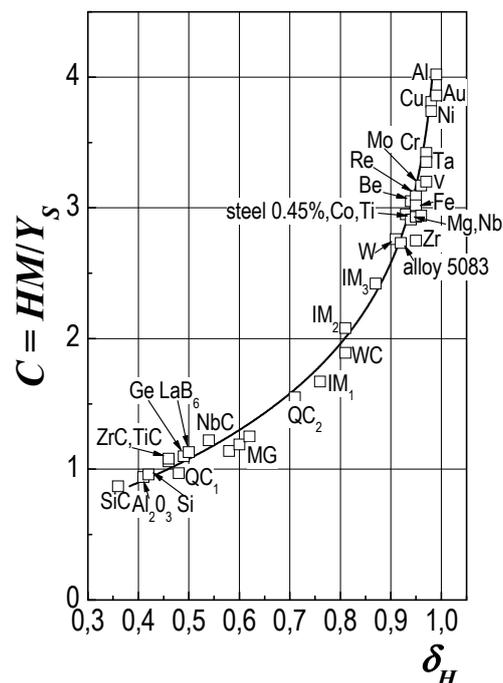
**Figure 3.** Relation between the Tabor parameter  $C = HM/Y_S$  and the plasticity characteristic  $\delta_H$ . Curve was constructed on the basis of Equation (13) for  $z = 0.38$  and  $\nu_S = 0.27$ .
