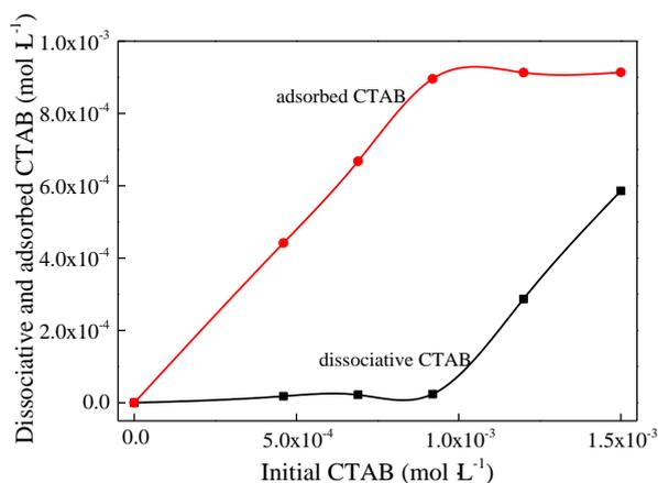
**Figure 5.** The dissociative and adsorbed CTAB after the hydrothermal reaction.
