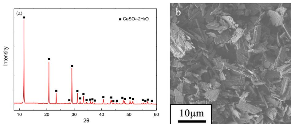
**Figure 1.** (a) XRD pattern and (b) SEM image of CaSO<sub>4</sub>·2H<sub>2</sub>O after calcination and hydration treatment.
