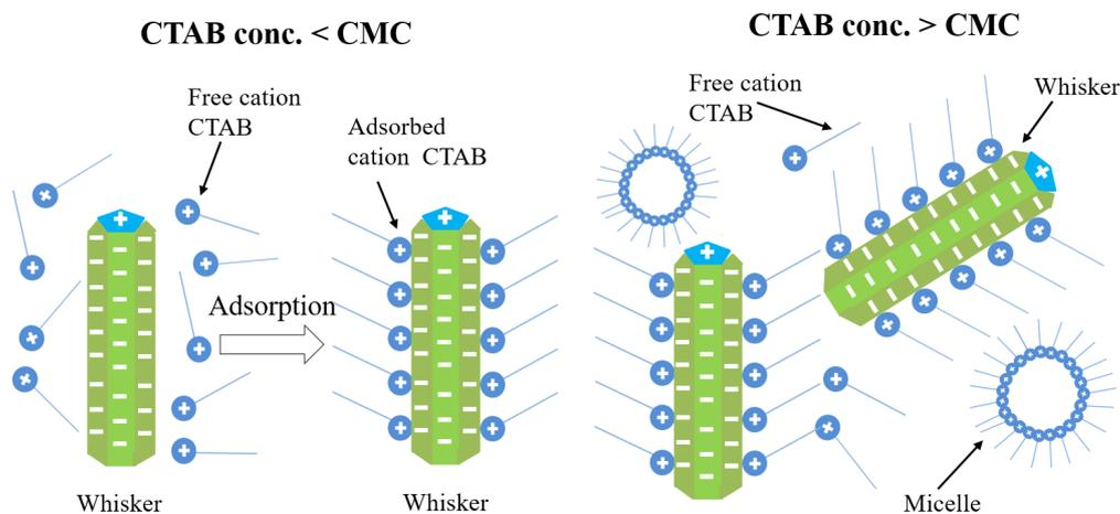
**Figure 6.** Adsorption sketch of CTAB on  $\alpha\text{-CaSO}_4\cdot 0.5\text{H}_2\text{O}$  whisker surfaces. CMC: critical micelle concentration.
