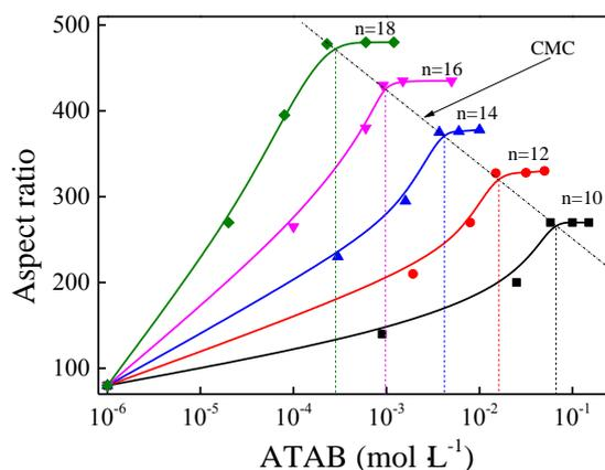
**Figure 7.** Influence of alkyl trimethyl ammonium bromides (C<sub>n</sub>H<sub>2n+1</sub>(CH<sub>3</sub>)<sub>3</sub>NBr, ATABs) on the aspect ratios of  $\alpha$ -CaSO<sub>4</sub>·0.5H<sub>2</sub>O whiskers.
