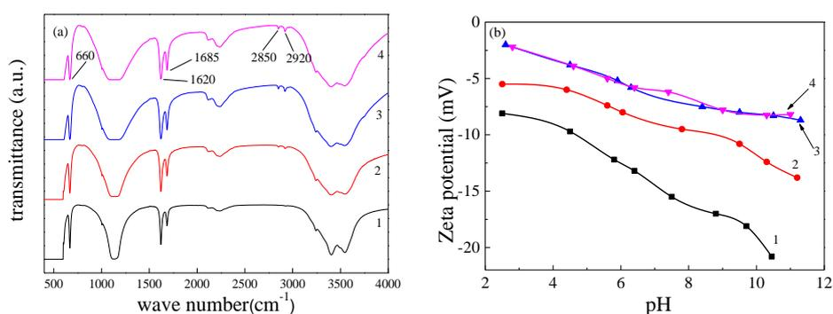
**Figure 4.** Variations of (a) Fourier transform infrared (FT-IR) spectra and (b) zeta potentials of  $\alpha$ -CaSO<sub>4</sub>·0.5H<sub>2</sub>O whiskers with the CTAB concentration (mol·L<sup>-1</sup>): 1—0, 2—1.0 × 10<sup>-4</sup>, 3—9.2 × 10<sup>-4</sup>, 4—1.5 × 10<sup>-3</sup>.
