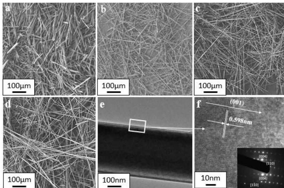
**Figure 2.** (a–d) SEM, (e) TEM, and (f) high-resolution TEM (HRTEM) images of  $\alpha$ -CaSO<sub>4</sub>·0.5H<sub>2</sub>O whiskers CTAB (cetyl trimethyl ammonium bromide, C<sub>16</sub>H<sub>33</sub>(CH<sub>3</sub>)<sub>3</sub>NBr) (mol·L<sup>-1</sup>): (a) 0; (b)  $1.0 \times 10^{-4}$ ; (c,e,f)  $9.2 \times 10^{-4}$ ; (d)  $1.5 \times 10^{-3}$ .
