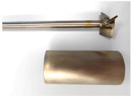
Figure S16. In-house small-scale high-shear granulator.
