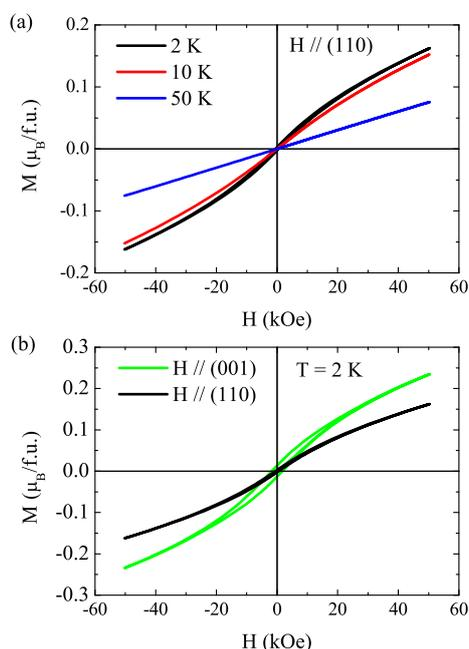
**Figure 4.** (Color online) (a) Isothermal magnetization measurement at different temperatures with the magnetic field along the [1 1 0]-direction; (b) Comparison of the magnetization at 2 K for magnetic fields along the [0 0 1]-direction and the [1 1 0]-direction, respectively.
