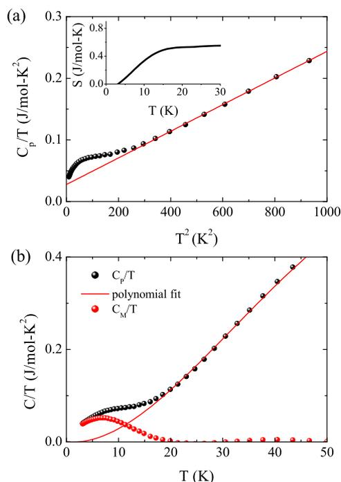
**Figure 5.** (Color online) (a)  $C_p/T$  vs.  $T^2$  plot at low temperatures. The red curve is a fit as described in the text. The inset shows the entropy change below 30 K; (b) Subtraction of the phonon component from  $C_p/T$  by a polynomial fit.
