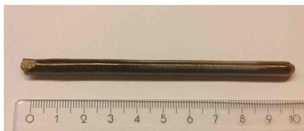
**Figure 1.** (Color online) A photo of the as-grown  $\text{LaSrCoO}_4$  crystal. The last  $\sim 6$  cm (on the right side) are single crystalline—i.e., roughly the part starting from number 4 on the ruler to somewhat below number 10 where the growth was finished.
