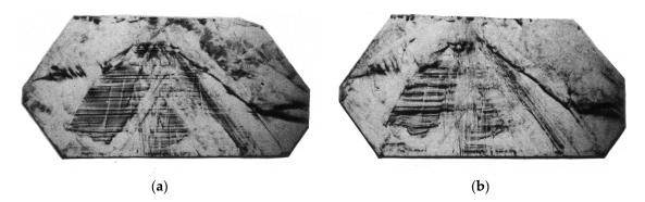
**Figure 6.** Synchrotron X-ray topographs of diamond B1—Image width 4 mm. Diffraction vector g pointing downwards. (**a**) 335 reflection,  $\lambda = 0.82$  Å,  $g \downarrow$ ; (**b**) 224 reflection,  $\lambda = 1.18$  Å,  $g \downarrow$ .
