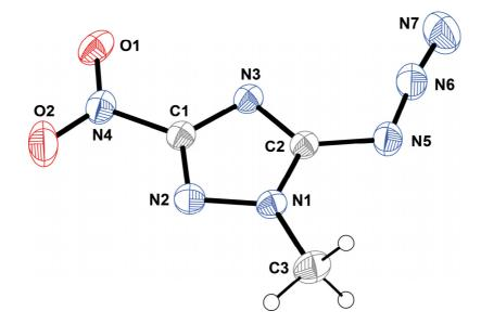
The geometry of the ring system is identical to the parent compound **1**. The N1–C3 bond is a true single bond with 1.463(4) Å.
