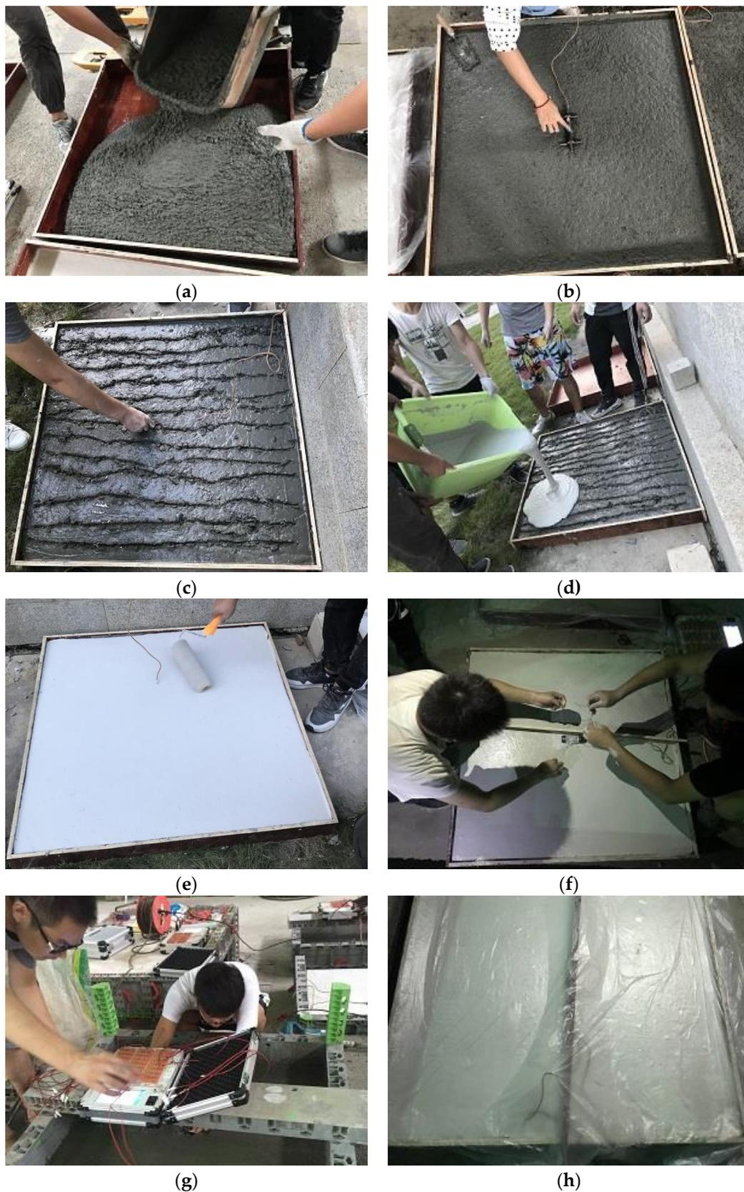
**Figure 6.** Experimental process: (a) pouring concrete; (b) placing embedded strain sensor; (c) surface processing; (d) pouring GRC material; (e) leveling the GRC surface; (f) placing surface strain sensors; (g) connecting the static strain tester; (h) covering film maintenance.
