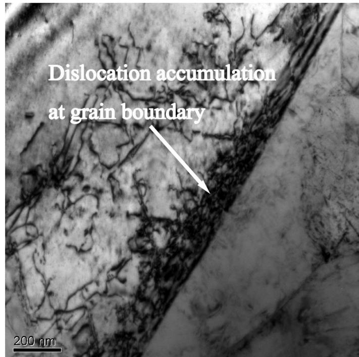
Figure 16. TEM image of specimen deformed at 960 °C.
