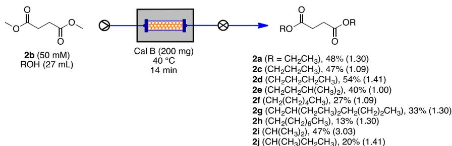
**Scheme 1.** Scope of the flow chemoenzymatic synthesis of dialkyl succinates **2a** and **2c–j** at 40 °C.
