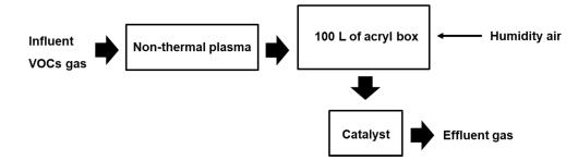
**Figure 8.** A schematic illustration of a non-thermal plasma (NTP)/catalyst hybrid reactor system for the VOCs decomposition from food waste.
