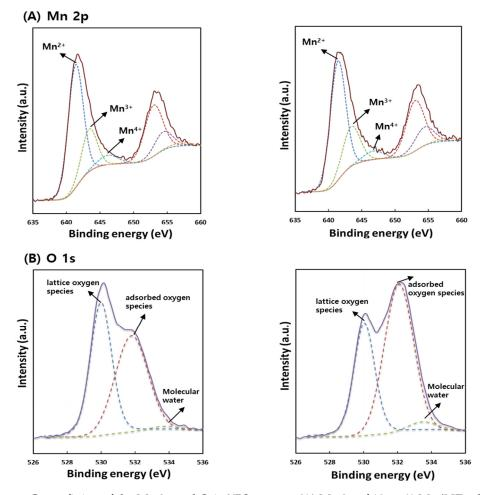
**Figure 2.** Curve fitting of the Mn 2p and O 1s XPS spectra. (**A**) Mn 2p of 10 wt.% Mn/NZ calcined at 350 °C and 550 °C, and (**B**) O 1s of 10 wt.% Mn/NZ calcined at 350 °C and 550 °C. Left: 10 wt.% Mn/NZ calcined at 350 °C, right: 10 wt.% Mn/NZ calcined at 550 °C.
