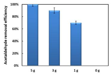
**Figure 4.** The effect of amount of catalysts (10 wt.% Mn/NZ) on the acetaldehyde oxidation in relative humidity 60%.
