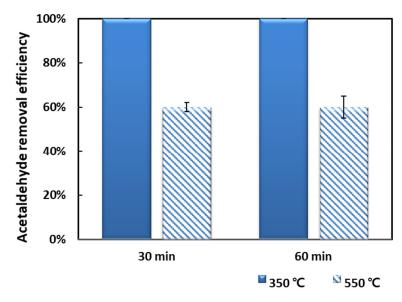
**Figure 6.** The effect of calcination temperature for the 10 wt.% Mn/NZ on the acetaldehyde oxidation. Relative Humidity: 60%, The amount of catalysts: 5 g.
