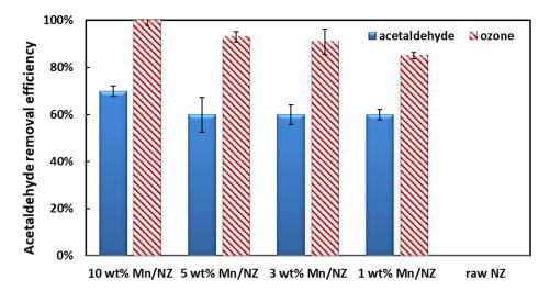
**Figure 3.** Acetaldehyde and ozone removal efficiencies of the Mn loaded NZ catalysts (1, 3, 5, and 10 wt.% Mn/NZ). Relative Humidity: 60%, The amount of catalysts: 1 g.
