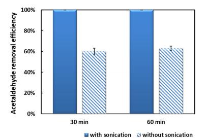
**Figure 5.** The effect of sonication on the catalytic activity of the 10 wt.% Mn/NZ for the acetaldehyde oxidation. Relative Humidity: 60%, The amount of catalysts: 5 g.
