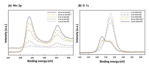
**Figure 1.** The Mn 2p and O 1s high resolved XPS spectra of 1, 3, 5 and 10 wt.% Mn/NZ (10 wt.% Mn/NZ \*: without sonication).
