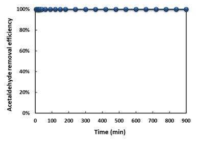
**Figure 7.** The long-term catalyst stability test for the acetaldehyde oxidation. Relative Humidity: 60%, The amount of catalysts: 5 g.
