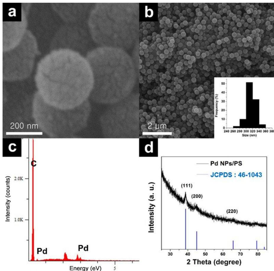
**Figure 2.** High- and low-resolution (a,b) SEM images of Pd/PS spheres. EDS spectrum (c) and XRD patterns (d) of Pd/PS spheres. The insert in (b) is the size distribution of Pd/PS spheres.
