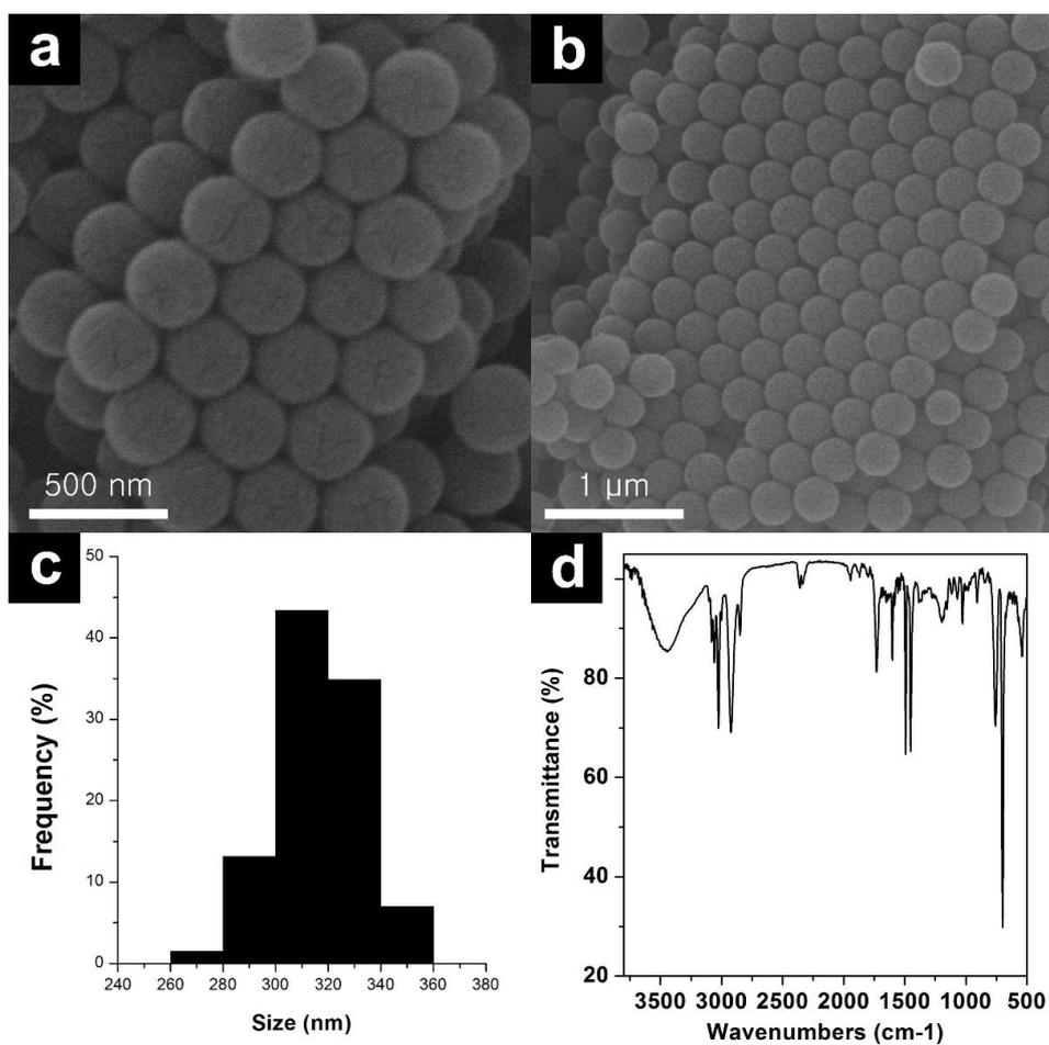
**Figure 1.** SEM images (a,b); size distribution (c) and FT-IR spectra (d) of PS spheres.
