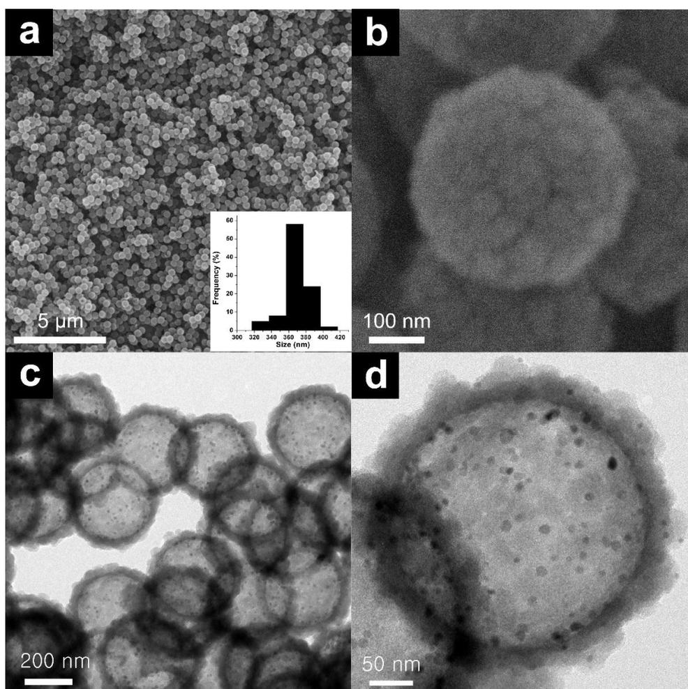
**Figure 5.** SEM images (a,b) and TEM image (c,d) of PdO/ZnO@mSiO<sub>2</sub> hybrid nanocatalyst. The insert in (a) is the size distribution of PdO/ZnO@mSiO<sub>2</sub> hybrid nanocatalyst.
