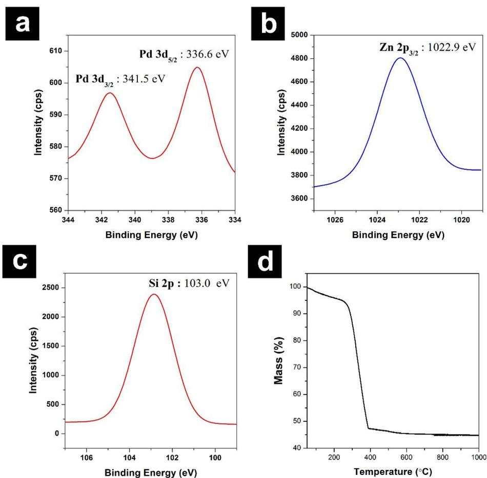
**Figure 6.** The XPS spectrums (a–c) of PdO/ZnO@mSiO<sub>2</sub> hybrid nanocatalyst and TGA curve (d) of PdO/ZnO@mSiO<sub>2</sub> hybrid nanocatalyst.
