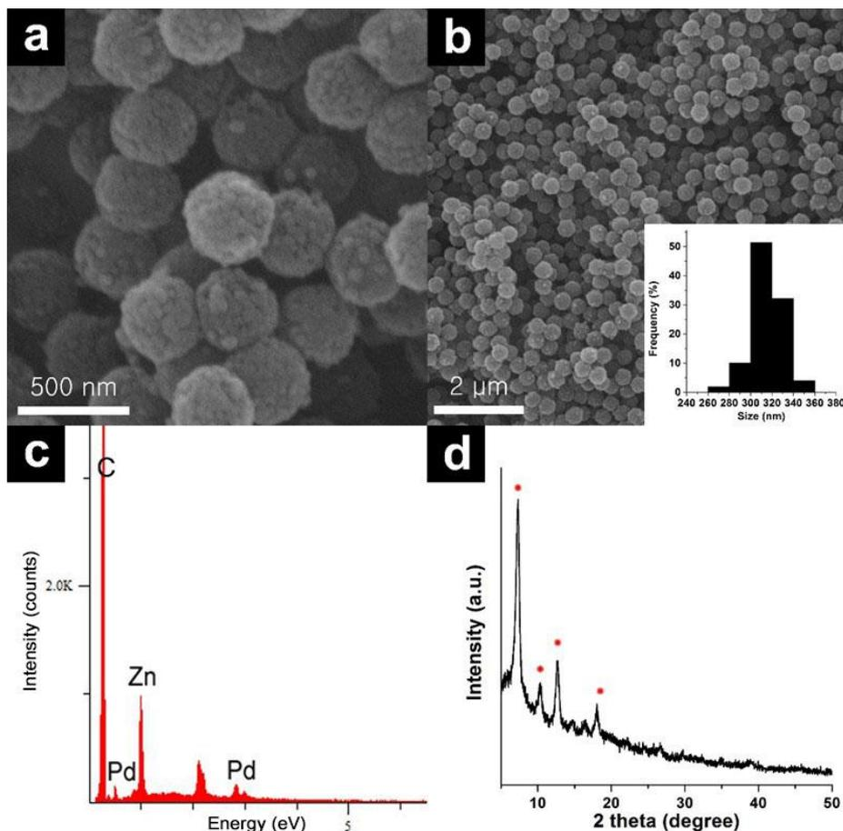
**Figure 3.** SEM images (a,b); EDS spectrum (c) and XRD patterns (d) of Pd/PS@ZIF-8 core-shell nanocomposites. The insert in (b) is the size distribution of Pd/PS@ZIF-8 core-shell nanocomposites.
