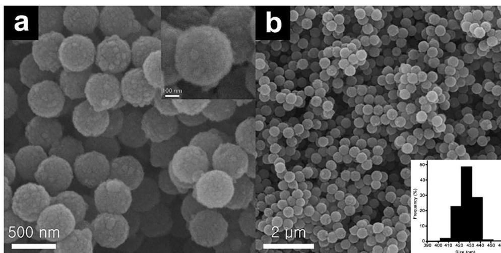
**Figure 4.** SEM images of Pd/PS@ZIF-8@mSiO<sub>2</sub> nanocomposites (a,b). The insert in (a) is high-resolution SEM image and the insert in (b) is the size distribution of Pd/PS@ZIF-8@mSiO<sub>2</sub> nanocomposites.
