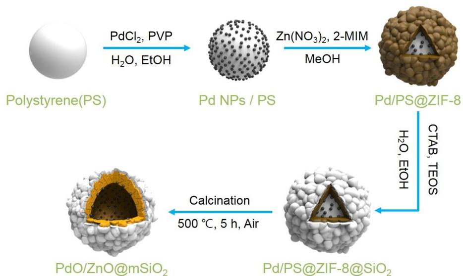
**Scheme 1.** Synthetic route for the PdO/ZnO@mSiO<sub>2</sub> hybrid nanocatalyst.
