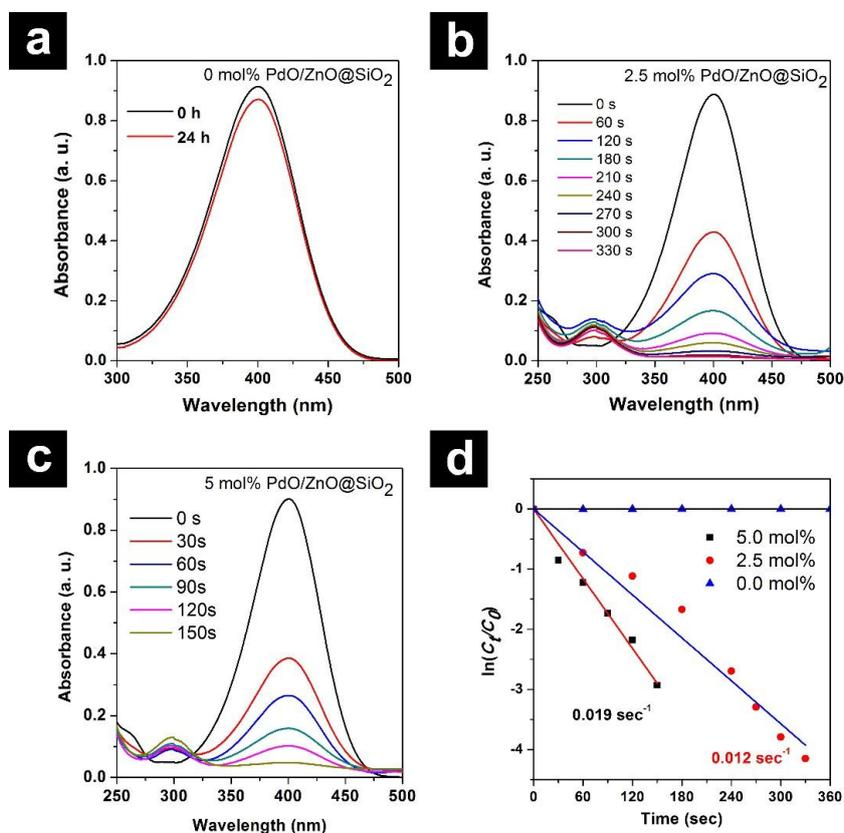
**Figure 7.** Time-dependent UV-vis absorption spectra for the reduction of 4-NP over different amount of catalyst, 0 mol % (a); 2.5 mol % (b); 5 mol % (c); and Plot of  $\ln(C_t/C_0)$  versus time for the reduction of 4-NP with different amount of catalyst (d).
