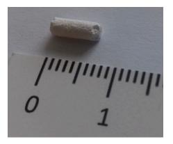
Figure 5. Homemade catalyst extrudate pellet.
