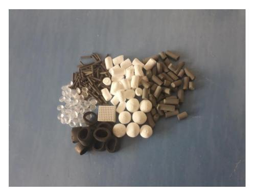
Figure 3. Different catalyst morphologies.
