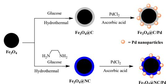
**Scheme 1.** Synthesis of  $\text{Fe}_3\text{O}_4\text{/C}$ /Pd and  $\text{Fe}_3\text{O}_4\text{/NC}$ /Pd catalysts.
