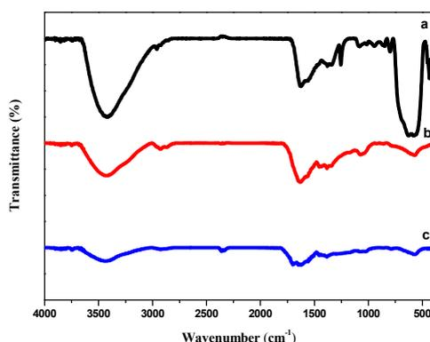
**Figure 1.** Fourier-transform infrared (FTIR) spectra of (a)  $\text{Fe}_3\text{O}_4$ , (b)  $\text{Fe}_3\text{O}_4@\text{NC}$ , and (c)  $\text{Fe}_3\text{O}_4@\text{NC}/\text{Pd}$ .
