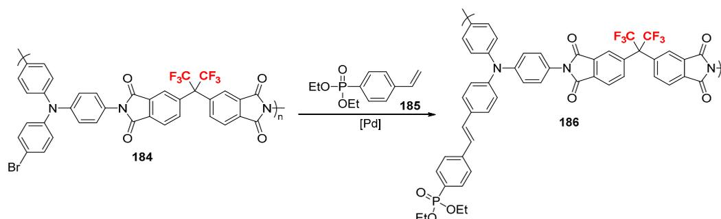
**Scheme 38.** Synthesis of multifunctional polymers for photorefractive applications by the Mizoroki-Heck reactions.
