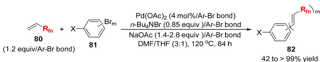
**Scheme 16.** The Mizoroki-Heck reactions of aromatic bromides and polybromides with fluororous alkenes.
