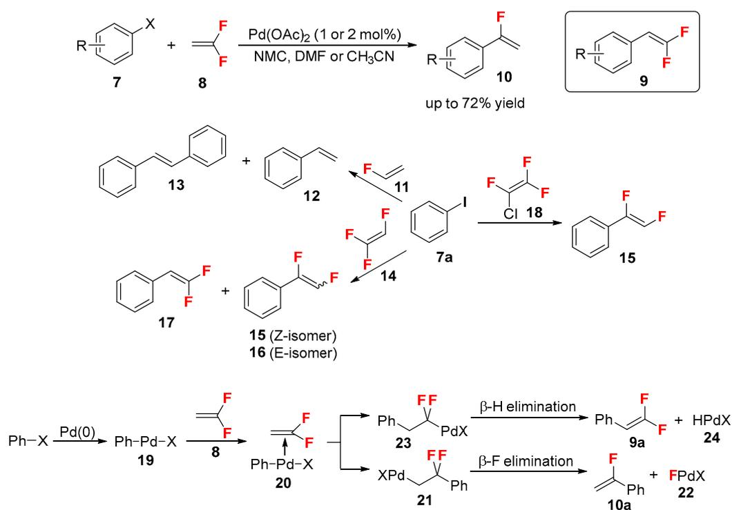
Scheme 2. Pd-catalyzed reactions of aromatic halides with fluoroolefins.
