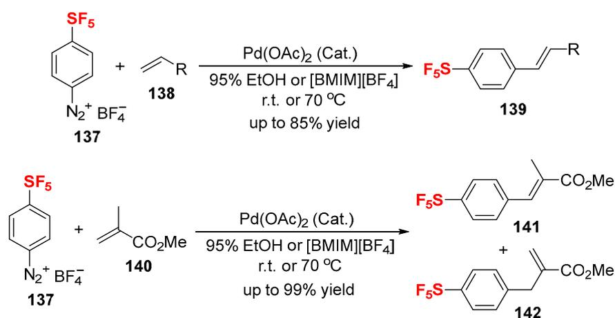
**Scheme 28.** The Heck-type reactions of 4-(pentafluorosulfonyl)benzenediazonium tetrafluoroborate.
