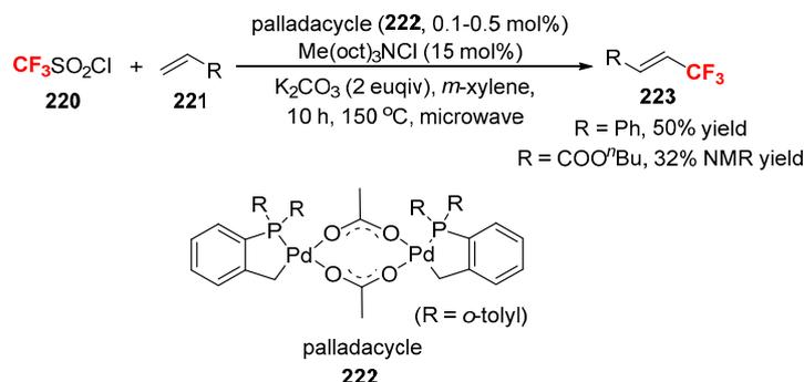
**Scheme 44.** Pd-catalyzed desulfitative Mizoroki-Heck type reactions of trifluoromethanesulfonyl chlorides with terminal alkenes.
