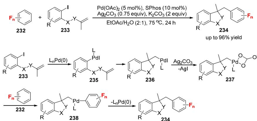
**Scheme 47.** Pd-catalyzed Heck/intermolecular C–H bond functionalization for the synthesis of alkylated polyfluoroarene derivatives.
