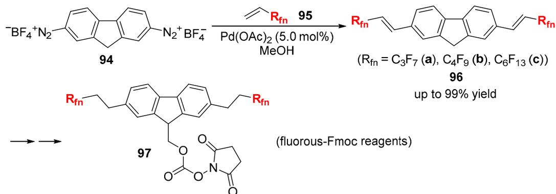
**Scheme 19.** Multi-gram scale and divergent preparation of fluorous-Fmoc reagents via the Mizoroki-Heck reactions.
