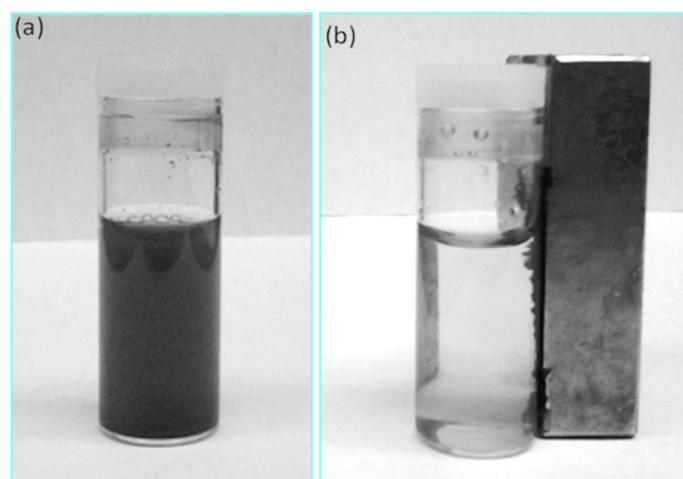
**Figure 7.** (a) Image of the reaction mixture using 0.3 mol % Pd/Fe<sub>3</sub>O<sub>4</sub>/G catalyst after reaction; (b) Separation of spent catalyst from reaction mixture using a simple magnet. Reprinted from [128]. Copyright (2015), with permission from Elsevier.
