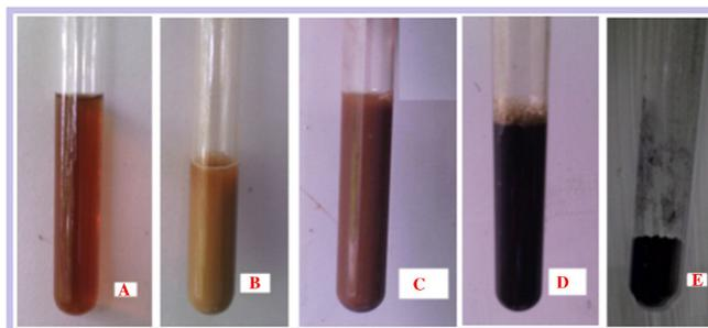
**Figure 4.** Photograph of (A) hearth wood extract of *A. lakoocha* Roxb in water; (B) solution A with cellulose; (C) Solution B with  $PdCl_2$ ; (D) Solution C after 15 min warming in heating bath at 60 °C; (E) solid recyclable  $Pd(0)$  NPs@cellulose. Reprinted from [108]. Copyright (2015), with permission from Elsevier.
