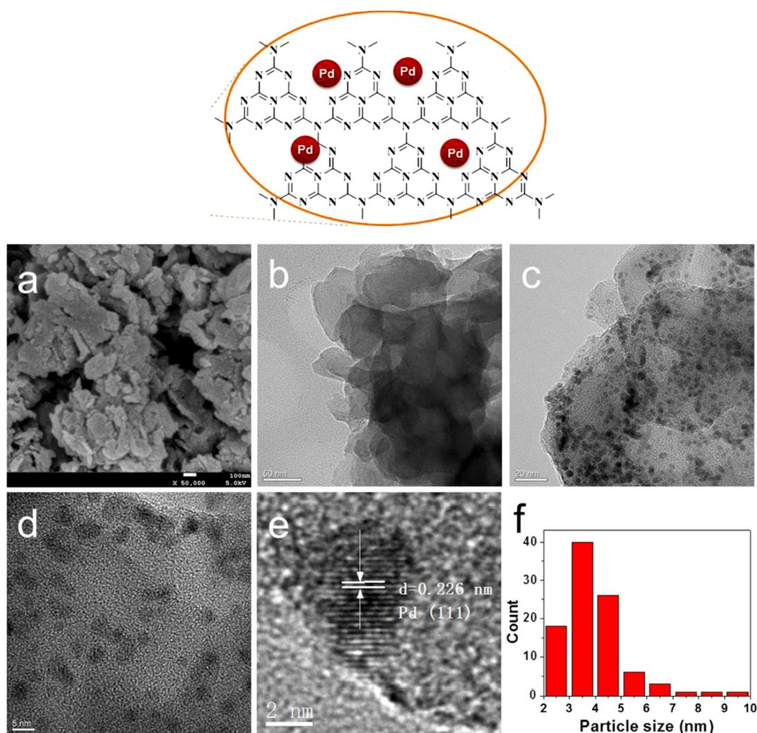
**Figure 17.** Top: Pd NPs, supported on the  $\gamma\text{-C}_3\text{N}_4$  surface. Bottom: SEM image of  $\gamma\text{-C}_3\text{N}_4$  (a); TEM images of  $\gamma\text{-C}_3\text{N}_4$  (b); and Pd/ $\gamma\text{-C}_3\text{N}_4$  (c); HRTEM images of Pd/ $\gamma\text{-C}_3\text{N}_4$  (d,e); and size distribution of Pd NPs (f) (Reproduced from [148]. Copyright (2015), with permission of Springer).
