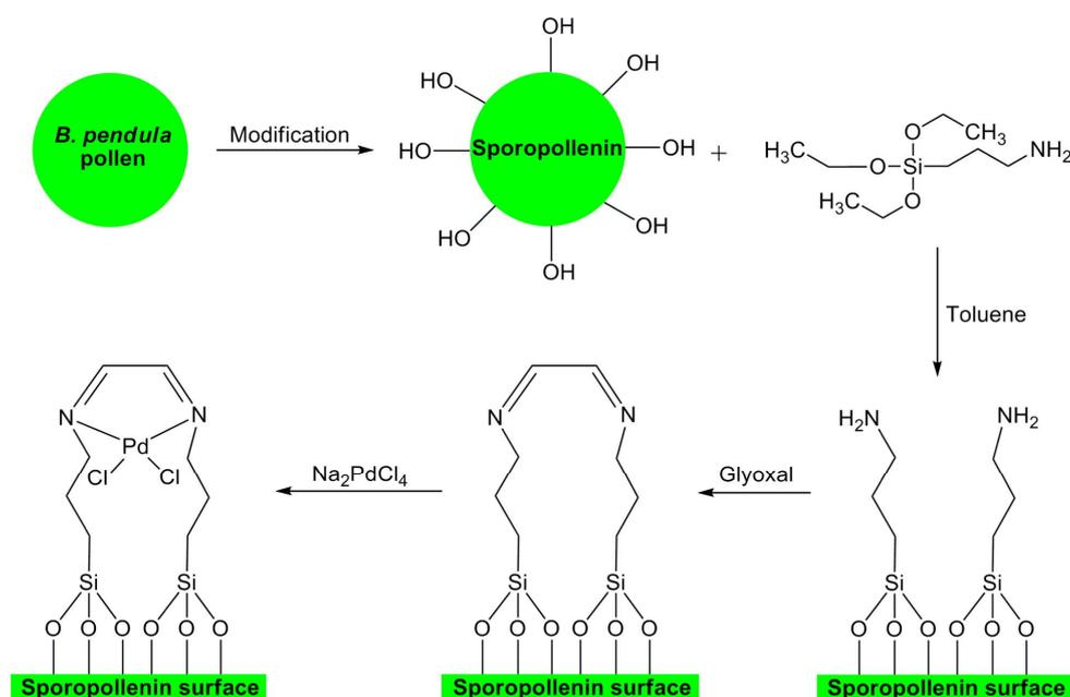
**Scheme 52.** Design of sporopollenin microcapsule supported Pd(II) catalyst. Reprinted from [109]. Copyright (2016), with permission from Elsevier.
