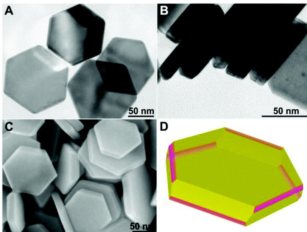
**Figure 25.** (A) Top-view; and (B) side-view TEM; (C) SEM images; and (D) sketch of the Pd hexagonal nanoplates. Yellow and pink represent the {111} and {100} planes, respectively. Reprinted from [180]. Copyright (2015), with permission from Royal Society of Chemistry.
