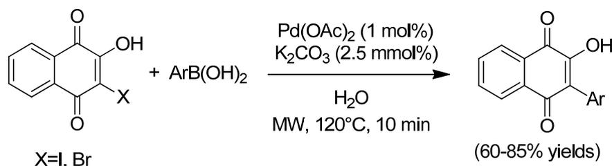
**Scheme 3.** Synthesis of 3-aryl-2-hydroxy-1,4-naphthoquinone analogues.
