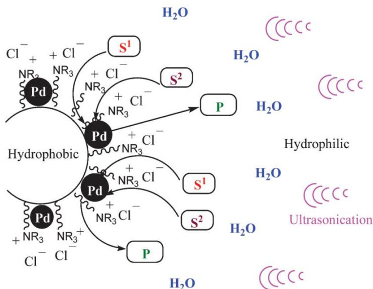
**Figure 11.** A schematic diagram of the reaction outline on the catalyst surface; S<sup>1</sup> = aryl halide, S<sup>2</sup> = phenylboronic acid and P = product (Reproduced from [137]. Copyright (2013), with permission from Royal Society of Chemistry).
