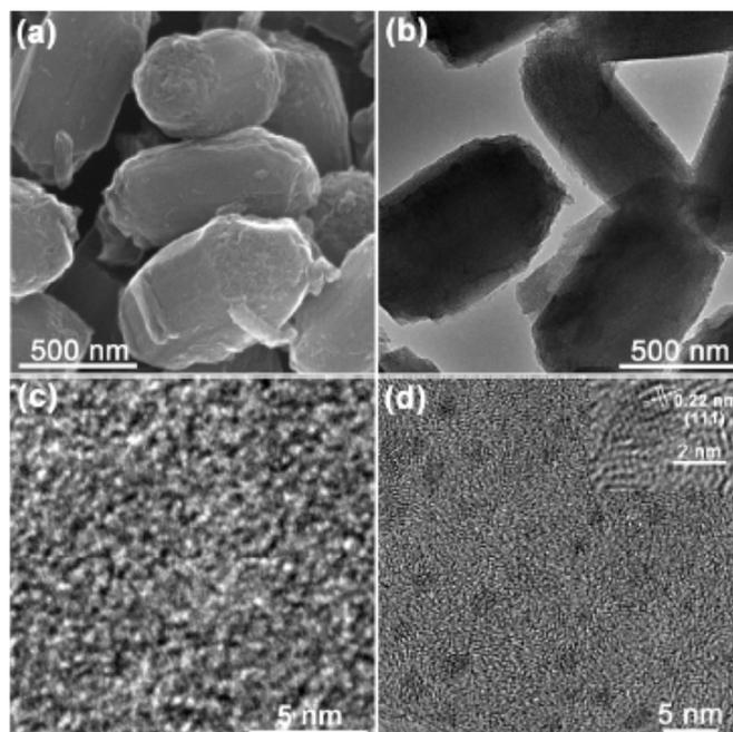
**Figure 15.** Electron microscope images of Pd@CMK-3. (a) SEM image; (b) TEM image; (c) typical HRTEM image; (d) HRTEM image of the sample after 30 min irradiation (300 keV), and the inset showing the lattice fringe of a typical Pd NP (Reproduced from [143]. Copyright (2014), with permission of Springer).
