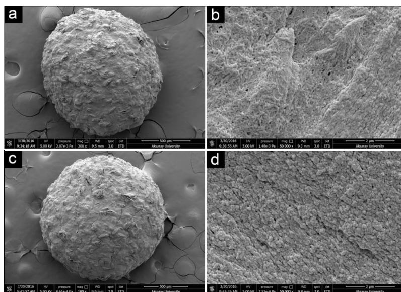
**Figure 1.** Scanning electron microscopy (SEM) images of (a,b) cross linked-chitosan-cellulose composite micro beads; (c,d) green chitosan/cellulose-Pd(II) catalyst. Reprinted from [100]. Copyright (2016), with permission from Elsevier.
