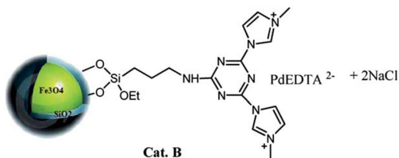
**Figure 14.** General structure of SPION-A-Pd(EDTA) nanocatalyst. (Reproduced from [142]. Copyright (2014), with permission from Royal Society of Chemistry).
