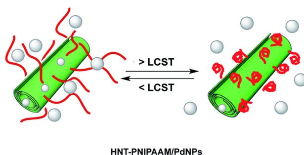
**Figure 3.** Sketch representation of the swelling behavior of HNT-PNIPAAm/Pd nanoparticles at the critical solution temperature (32 °C). Reprinted from [105]. Copyright (2016), with permission from Royal Society of Chemistry.
