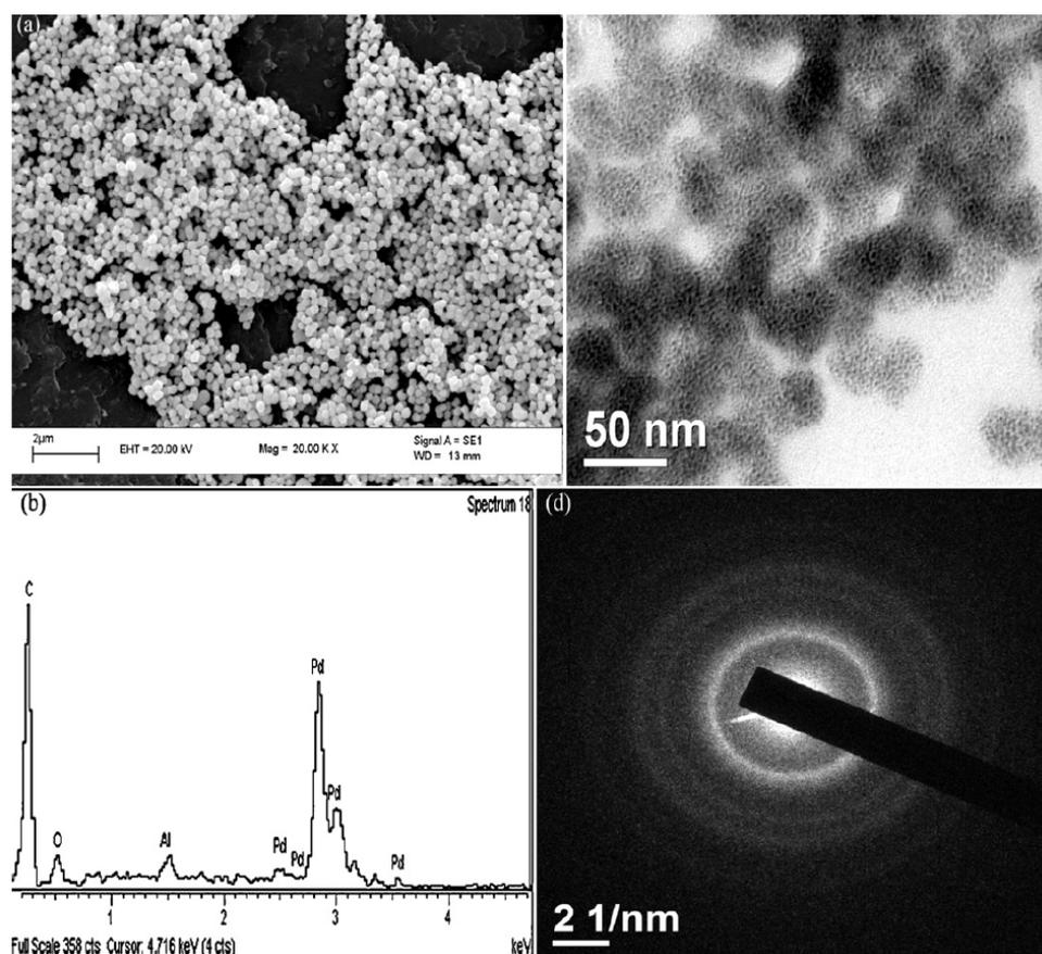
**Figure 16.** SEM with EDX (a,b) and TEM image with Selected Area Electron Diffraction (SAED); (c,d) of ferrite magnetic nanoparticles (Pd–CoFe<sub>2</sub>O<sub>4</sub> MNPs) (Reproduced from [146]. Copyright (2012), with permission from Elsevier).
