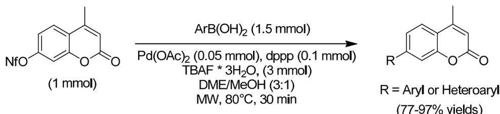
**Scheme 7.** SMC applied to 7-substituted coumarins preparation.
