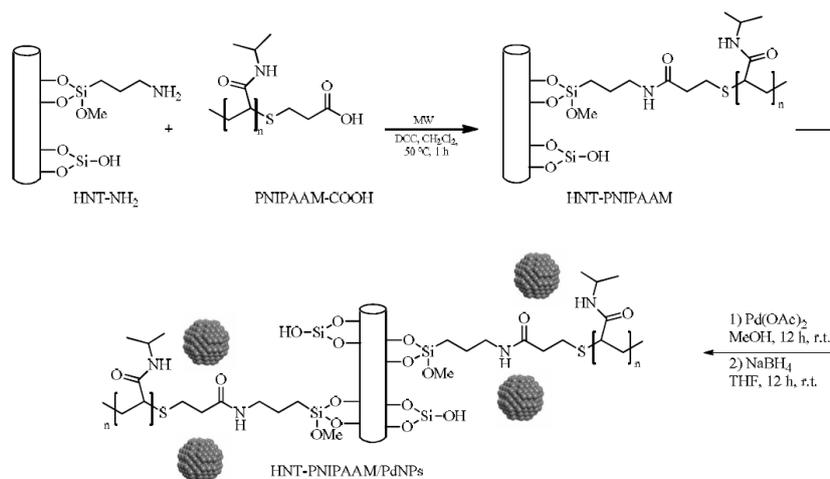
**Scheme 50.** Representation of the synthesis of Pd nanoparticles immobilised into Poly(*N*-isopropylacrylamide) (PNIPAAm) previously grafted onto halloysite nanotubes (HNT). Reprinted from [105]. Copyright (2016), with permission from Royal Society of Chemistry.
