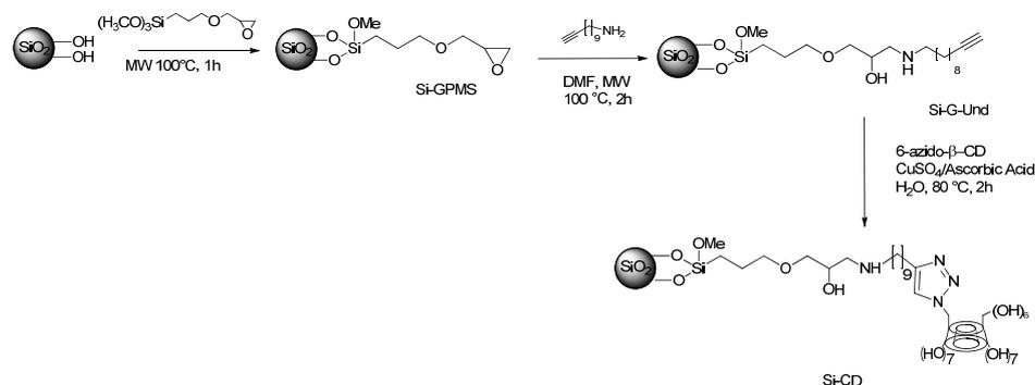
**Scheme 47.** Synthetic procedure for the preparation of Si-cyclodextrin [102].
