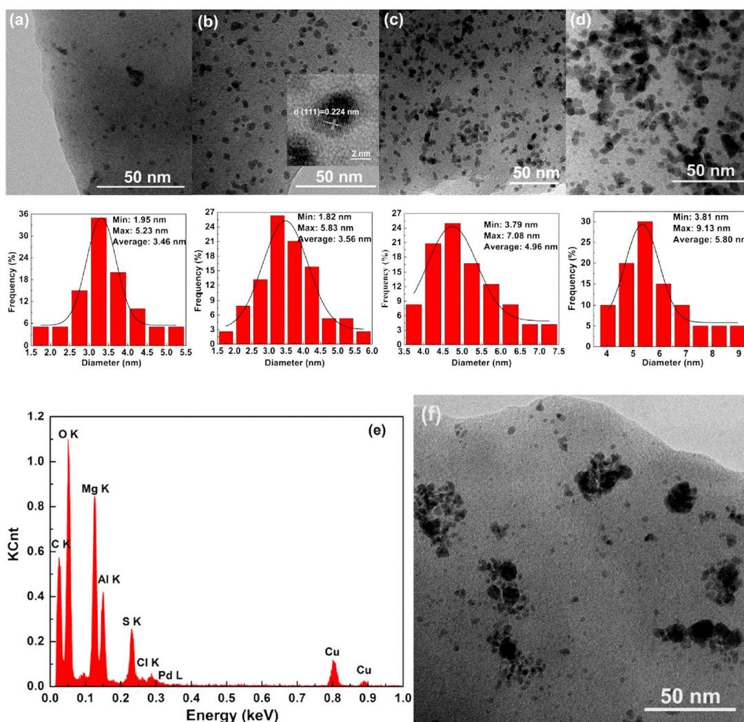
**Figure 18.** TEM images and corresponding size distributions of the Pd<sub>0.005</sub>/SDS-LDHs (Sodium Dodecylsulfonate-Layered double hydroxides) (a); Pd<sub>0.02</sub>/SDS-LDHs (b) (HRTEM images (inset)); Pd<sub>0.05</sub>/SDS-LDHs (c); and Pd<sub>0.10</sub>/SDS-LDHs (d); EDS profile of the Pd<sub>0.02</sub>/SDS-LDHs (e); Pd<sub>0.02</sub>/SDS-LDHs prepared in the absence of US (f). (Reproduced from [149]. Copyright (2016), with permission from Springer).
