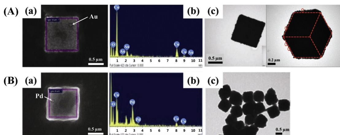
**Figure 8.** (a) SEM; (b) EDXS; and (c) TEM images of (A) Au and (B) Pd nanoparticle decorated Cu<sub>2</sub>O microcubes. Reprinted from [133]. Copyright (2014), with permission from Elsevier.
