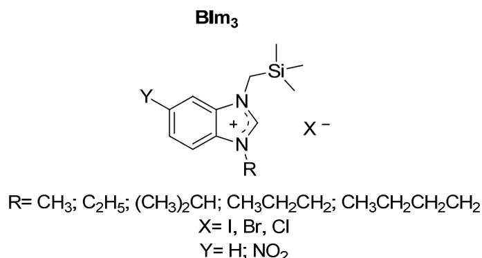
**Scheme 37.** General structure of benzimidazole salts which contain trimethylsilylmethyl substituent (**Bim<sub>3</sub>**).
