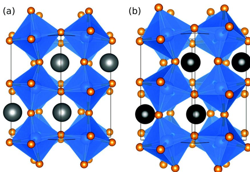
**Figure 10.** Crystal structures for (a)  $\text{LaFeO}_3$ ; and (b)  $\text{YFeO}_3$ . The A site cations are displayed as grey spheres and  $\text{FeO}_6$  octahedra in blue. Reprinted from [135]. Copyright (2013), with permission from Royal Society of Chemistry.
