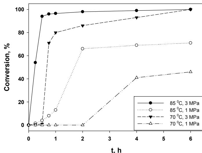
**Figure 5.** Kinetics of phenol hydrogenation in water in the presence of G3-dendr-SiO<sub>2</sub>-Ru at substrate/Ru = 377. Reaction conditions are:  $m(\text{PhOH}) = V(\text{H}_2\text{O})$ .
