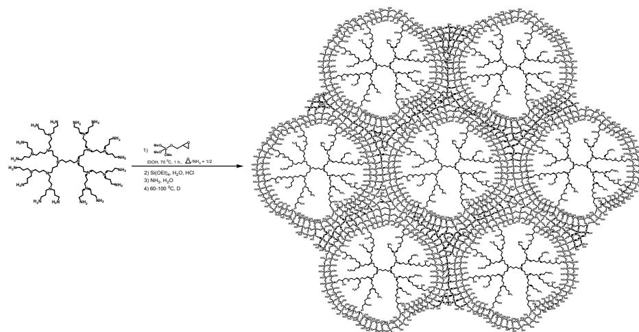
**Scheme 2.** The synthesis of hybrid G3-dendr-SiO<sub>2</sub> material.
