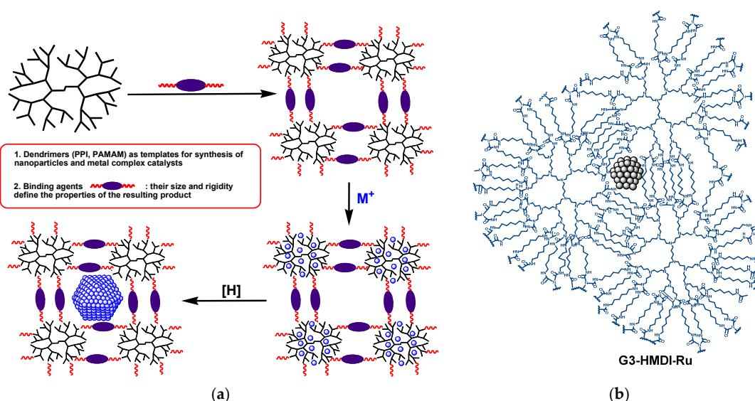
**Scheme 1.** (a) Approach for synthesis of nanoheterogeneous catalysts, based on dendrimer cross-linked networks [56–59,61]; (b) representative structure for Ru nanocatalysts, based on PPI dendrimers of the 3rd generation, cross-linked with hexamethylene diisocyanate (HMDI).
