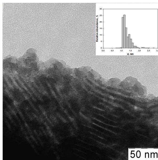
**Figure 3.** G2-dendr-*meso*-SiO<sub>2</sub>-Ru catalyst: TEM microphotography and particles size distribution.
