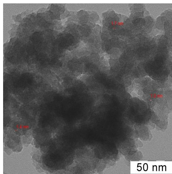
**Figure 2.** TEM microphotography of hybrid G3-dendr-SiO<sub>2</sub> material.
