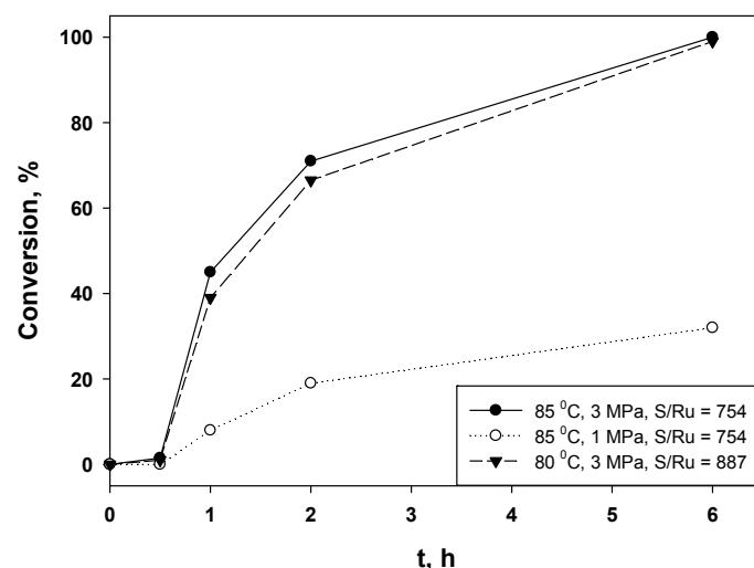
**Figure 6.** Kinetics of phenol hydrogenation in water in the presence of G3-dendr-SiO<sub>2</sub>-Ru at substrate/Ru = 754–887. Reaction conditions are:  $m(\text{PhOH}) = V(\text{H}_2\text{O})$ .
