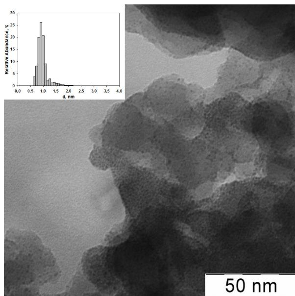
**Figure 4.** G3-dendr-SiO<sub>2</sub>-Ru catalyst: TEM microphotography and particles size distribution.
