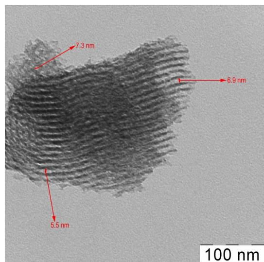
**Figure 1.** Transmission electron microscopy (TEM) microphotography of G2-dendr-meso-SiO<sub>2</sub> material.
