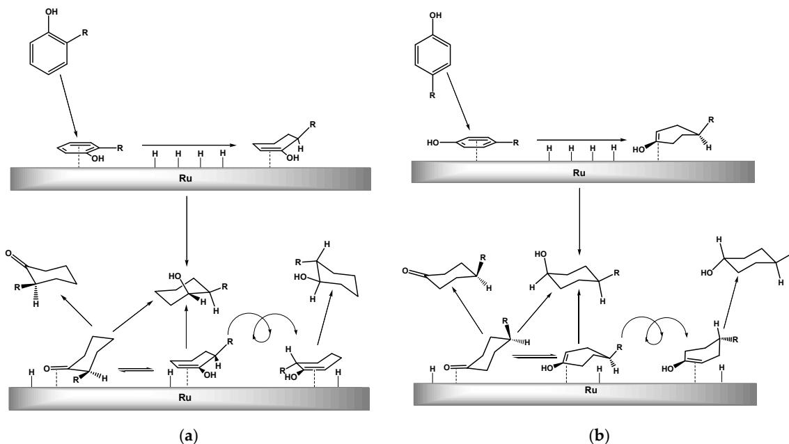
**Figure 8.** Possible ways for *cis*- and *trans*-product formation from *ortho*- and *para*-alkyl-substituted phenols. (a) *ortho*-isomers, (b) *para*-isomers.
