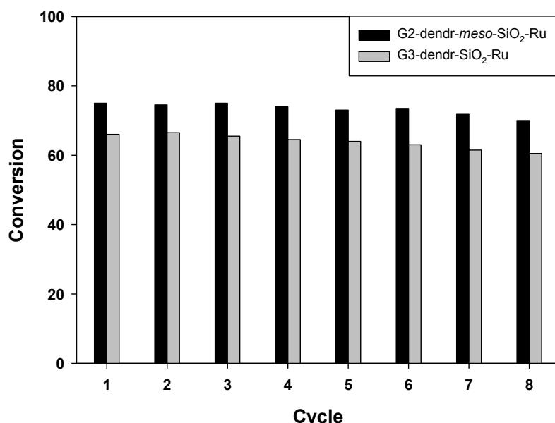
**Figure 10.** Recycling of porous silica-immobilized dendrimer-based Ru catalysts in phenol hydrogenation. Reaction conditions are: 5 mg of catalyst, 300 mg of phenol, 300  $\mu$ L of water, at 80  $^{\circ}$ C, 3 MPa of H<sub>2</sub> for 2 h. PhOH/Ru  $\approx$  1843 for G2-dendr-meso-SiO<sub>2</sub>-Ru and 887 for G3-dendr-SiO<sub>2</sub>-Ru.
