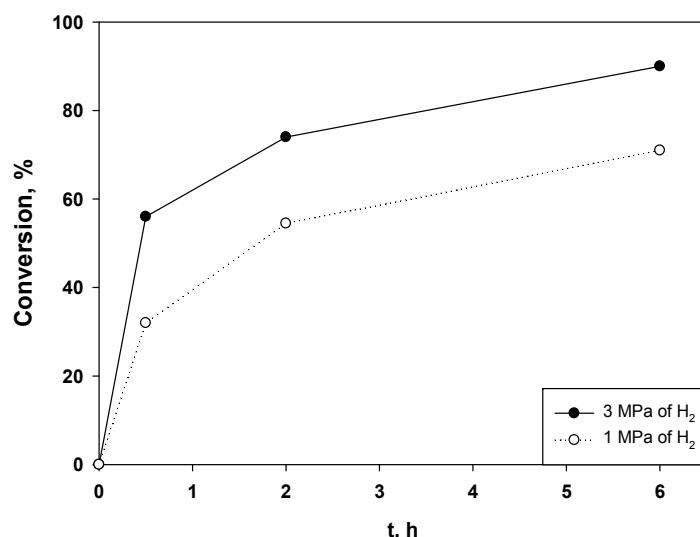
**Figure 7.** Hydrogenation of phenol in water in the presence of G2-dendr-*meso*-SiO<sub>2</sub>-Ru. Reaction conditions are: S/Ru = 1843, at 80 °C,  $m(\text{substr.}) = V(\text{H}_2\text{O})$ .
