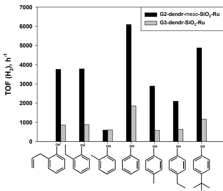
**Figure 9.** Hydrogenation of alkyl-substituted phenols in the presence of porous silica-immobilized dendrimer-based Ru catalysts. Reaction conditions are: at 80 °C, 3 MPa of H<sub>2</sub>, V(substrate) = V(H<sub>2</sub>O).
