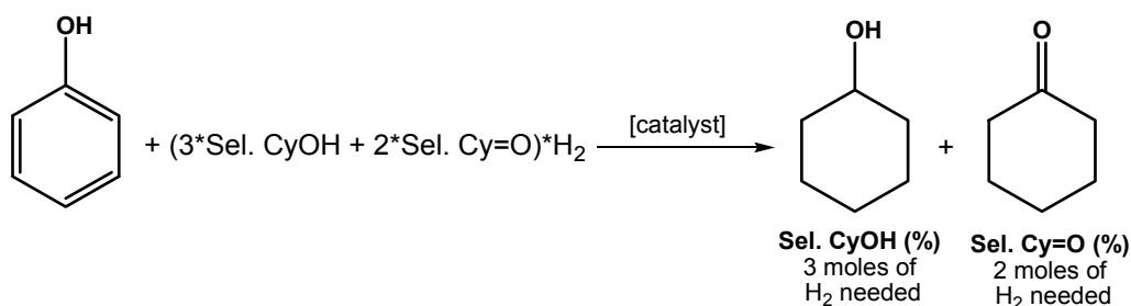
**Scheme 4.** Typical illustration for calculation of hydrogen consumed.
