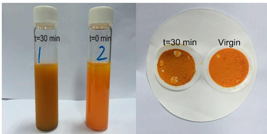
**Fig. S5.** Color change of BiOI suspension during the degradation process. ( $[\text{CBZ}]_0 = 5.0 \mu\text{M}$ ,  $[\text{PMS}]_0 = 4.0 \text{ mM}$ ,  $[\text{BiOI}]_0 = 1.0 \text{ g}\cdot\text{L}^{-1}$ ,  $\text{pH} = 7.0$ ,  $24 \text{ }^\circ\text{C}$ )
