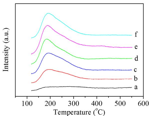
**Figure 7.** NH<sub>3</sub>-TPD (temperature-programmed desorption) profiles of V/SBA catalysts with different vanadium content. (a) 1% V/SBA; (b) 3% V/SBA; (c) 5% V/SBA; (d) 7% V/SBA; (e) 7% V/MCM; (f) 11% V/SBA.
