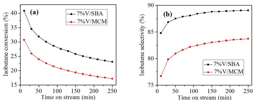
**Figure 9.** Conversion of isobutane (a) and selectivity to isobutene (b) as a function of time on stream for 7% V/SBA and 7% V/MCM catalysts at 570 °C.
