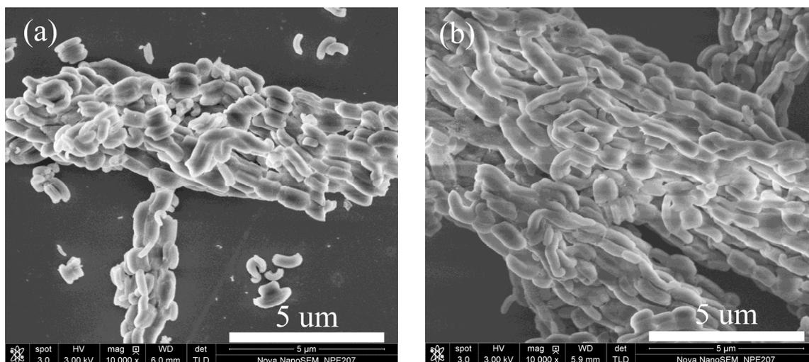
Figure 3. SEM images of (a) 3% V/SBA and (b) 7% V/SBA.
