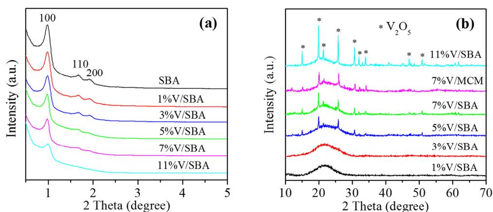
**Figure 1.** X-ray diffraction (XRD) patterns of SBA-15-supported vanadia catalysts in the small-angle region (a) and in the wide-angle region (b).
