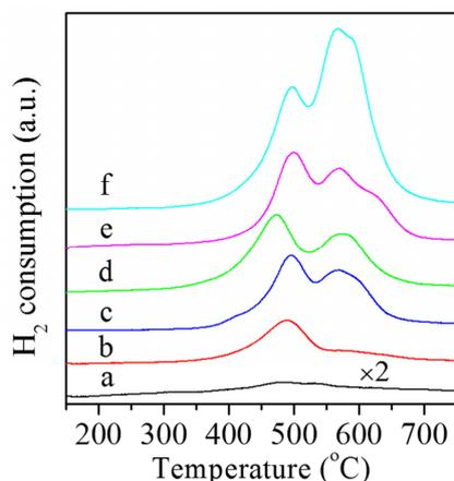
**Figure 6.** H<sub>2</sub>-TPR (temperature-programmed reduction) profiles of V/SBA catalysts with different vanadium content. (a) 1% V/SBA; (b) 3% V/SBA; (c) 5% V/SBA; (d) 7% V/SBA; (e) 7% V/MCM; (f) 11% V/SBA.
