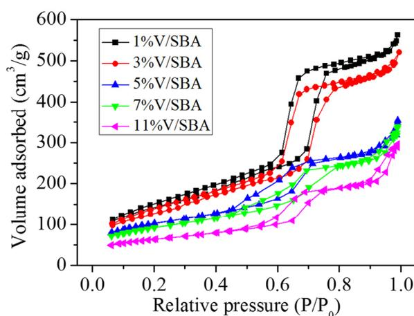
**Figure 2.** Nitrogen sorption isotherms of vanadia catalysts supported on SBA-15 (V/SBA) catalysts with different vanadium content.
