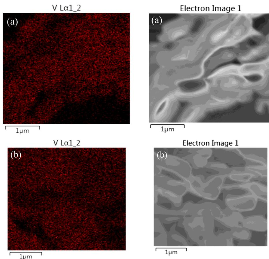
Figure 4. EDX elemental mapping of vanadia (V) (left column) and corresponding SEM images (right column) of (a) 3% V/SBA and (b) 7% V/SBA.
