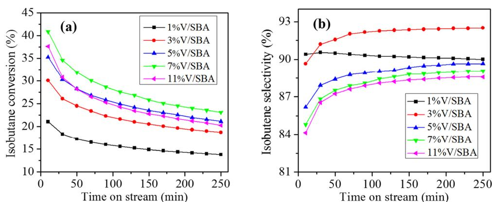
**Figure 8.** Conversion of isobutane (a) and selectivity to isobutene (b) as a function of time on stream for V/SBA catalysts at 570 °C.
