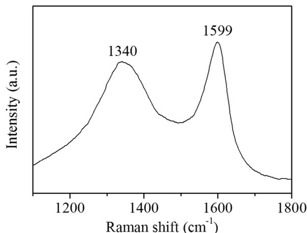
**Figure 10.** Raman spectrum of the spent 7% V/SBA catalyst after testing the dehydrogenation of isobutane with  $\text{CO}_2$  at 570 °C for 250 min.
