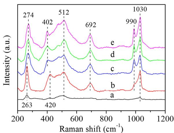
**Figure 5.** Raman spectra of V/SBA catalysts with different vanadium content. (a) 1% V/SBA; (b) 3% V/SBA; (c) 5% V/SBA; (d) 7% V/SBA; (e) 11% V/SBA.
