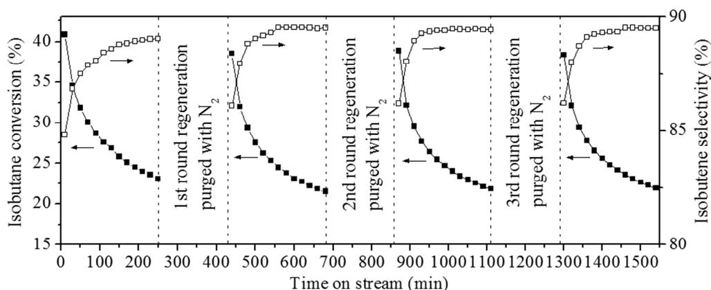
**Figure 11.** Regeneration of the 7% V/SBA catalyst at 550 °C. (■) conversion, (□) selectivity.
