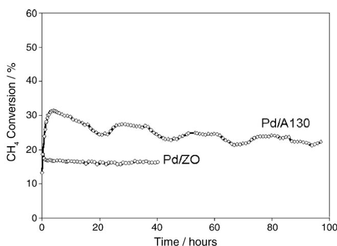
**Figure 7.** Methane conversion over time of Pd/ZrO<sub>2</sub> and Pd/Aerosil130 catalysts. Reaction conditions: 1.5% CH<sub>4</sub>; 6% O<sub>2</sub>; total flow = 90 cm<sup>3</sup>min<sup>-1</sup>, balanced in He; temperature = 325 °C; catalyst mass = 0.2 g. Reprinted with permission from [53]. Copyright © 2005 Elsevier.
