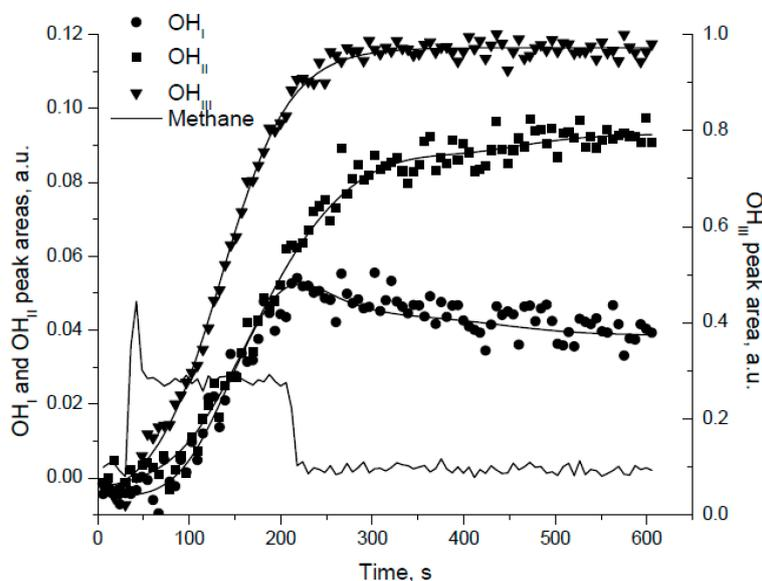
**Figure 11.** The normalized peak areas of different surface OH species generated during lean-CH<sub>4</sub>-O<sub>2</sub> reaction at 175 °C. Reproduced with permission from [30]. Copyright © 2004 Elsevier.
