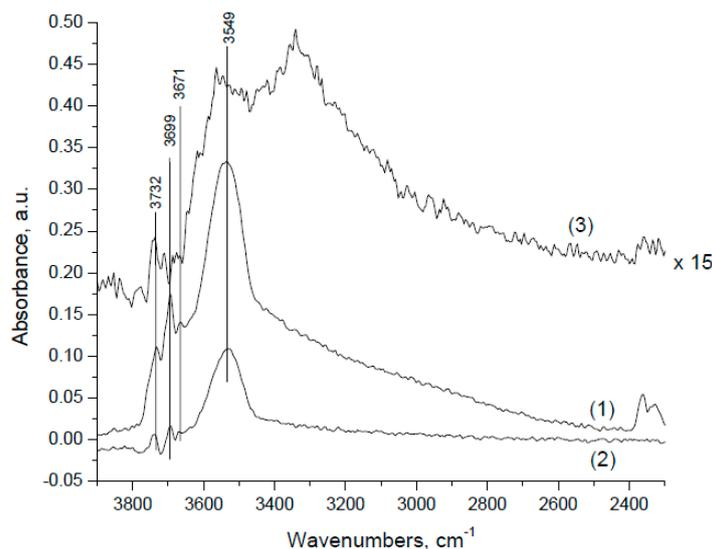
**Figure 10.** FTIR spectra at highest surface coverage and 350 °C on (1) PdO/Al<sub>2</sub>O<sub>3</sub> during CH<sub>4</sub>-O<sub>2</sub> reaction, (2) PdO/Al<sub>2</sub>O<sub>3</sub> and (3) Al<sub>2</sub>O<sub>3</sub> when injecting H<sub>2</sub>O pulses. Reproduced with permission from [30]. Copyright © 2004 Elsevier.
