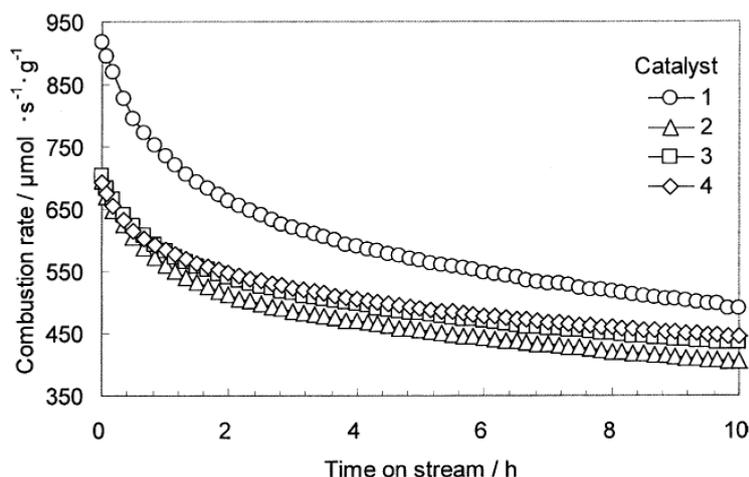
**Figure 15.** CH<sub>4</sub> combustion rate at 800 °C with time on stream. Combustion conditions: 1 vol.% CH<sub>4</sub>, 99 vol.% air, CH<sub>4</sub>/air flow = 450 L.h<sup>-1</sup>, catalyst weight = 0.3 g. Catalyst 1, 2, 3, and 4 represent 18.7 wt.% Pd, 18.4 wt.% Pd-1.6 wt.% Pt, 18.1 wt.% Pd-3.4 wt.% Pt, and 18.0 wt.% Pd-3.9 wt.% Pt over Al<sub>2</sub>O<sub>3</sub> catalysts. Reprinted with permission from [77]. Copyright © 2004 Elsevier.
