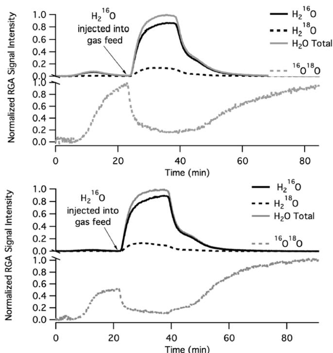
**Figure 12.** Oxygen exchange of (a) 3 wt.% Pd<sup>18</sup>O/Al<sub>2</sub><sup>16</sup>O<sub>3</sub> (top) and (b) 3 wt.% Pd<sup>18</sup>O/Mg<sup>16</sup>O (bottom) with catalyst supports in a flow of <sup>18</sup>O<sub>2</sub>/He at 400 °C. H<sub>2</sub><sup>16</sup>O was injected at some time to probe its effect on oxygen exchange. Reproduced with permission from [44]. Copyright ©2012 American Chemical Society.
