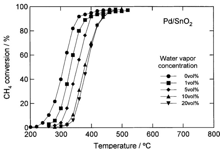
**Figure 5.** Catalytic combustion of CH<sub>4</sub> over 1.1 wt.% Pd/SnO<sub>2</sub> with different amounts of water added (vol.%). Reaction conditions: CH<sub>4</sub>, 1 vol.%; O<sub>2</sub>, 20 vol.%; H<sub>2</sub>O, 0–20 vol.%; N<sub>2</sub>, balance; GHSV 48,000 h<sup>-1</sup>. Reprinted with permission from [16]. Copyright© 2002 Elsevier.
