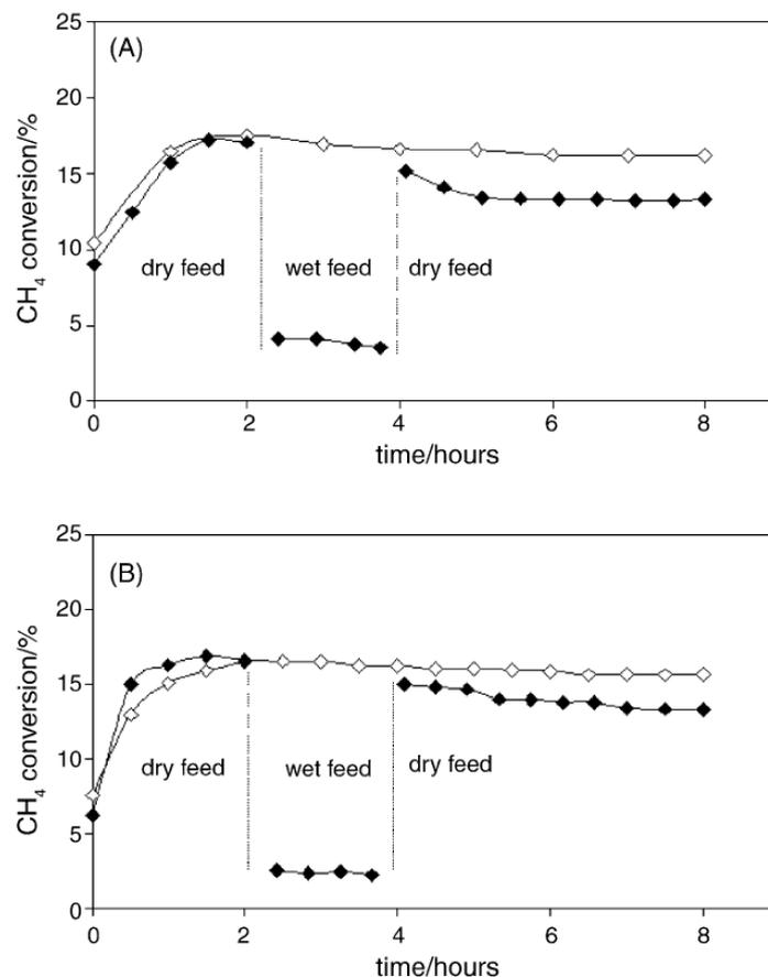
**Figure 8.** (A) Pd/Aerosil130 catalyst, (B) Pd/R972 catalyst. Reaction conditions: total flow = 90 cm<sup>3</sup> (STP) min<sup>-1</sup>, temperature = 325 °C; catalyst mass = 0.2 g. Open symbols: dry feed 1.5% CH<sub>4</sub>; 6% O<sub>2</sub>; balance He; closed symbol: wet feed 1.5% CH<sub>4</sub>; 6% O<sub>2</sub> with 3% H<sub>2</sub>O, balance He. Reproduced with permission from [53]. Copyright © 2005 Elsevier.
