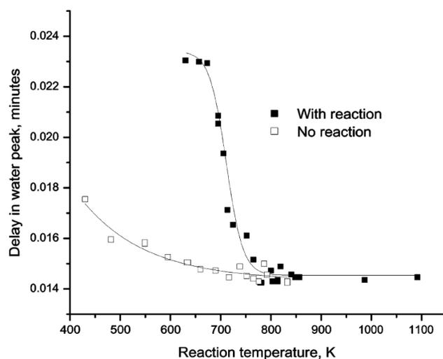
**Figure 2.** Delay in the H<sub>2</sub>O peak with respect to other products obtained by passing pulses of CH<sub>4</sub>/O<sub>2</sub>/He (closed square) and 1 vol.% O<sub>2</sub>/3.45 vol.% H<sub>2</sub>O/He (open square) over Pd/ZrO<sub>2</sub> at different temperatures. Reproduced with permission from [42]. Copyright © 2001 Elsevier.
