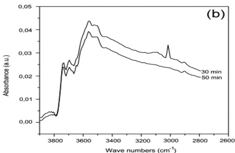
**Figure 9.** FTIR spectra of 5 wt.% Pd/Al<sub>2</sub>O<sub>3</sub> at 200 °C (a) during the CH<sub>4</sub>-O<sub>2</sub> reaction; (b) desorption when CH<sub>4</sub> was removed. Reproduced with permission from [35]. Copyright© 2007 Elsevier.
