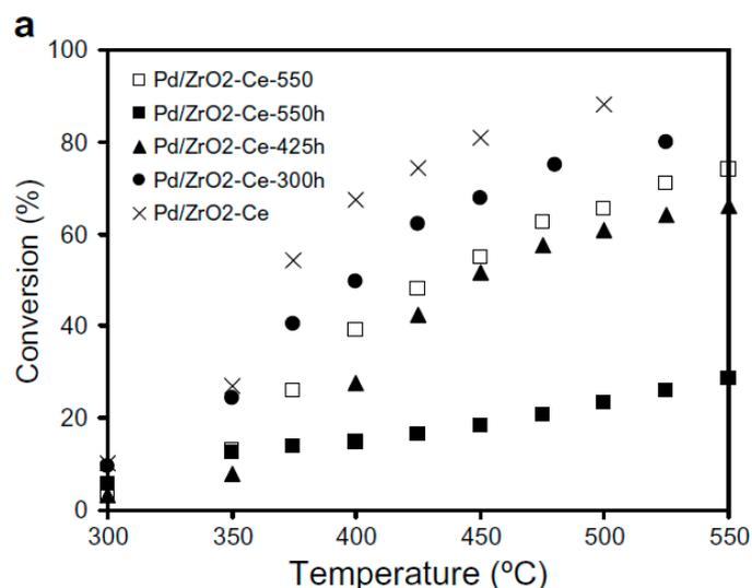
**Figure 4.** CH<sub>4</sub> conversion over fresh 1 wt.% Pd/ZrO<sub>2</sub>-Ce catalyst compared to 1 wt.% Pd/ZrO<sub>2</sub>-Ce thermally aged in air at 550 °C (Pd/ZrO<sub>2</sub>-Ce-550) and hydrothermally aged at different temperatures in 2% H<sub>2</sub>O/air (identified as Pd/ZrO<sub>2</sub>-Ce-TTT where TTT is the aging temperature in °C). Reproduced with permission from [49]. Copyright© 2008 Elsevier.
