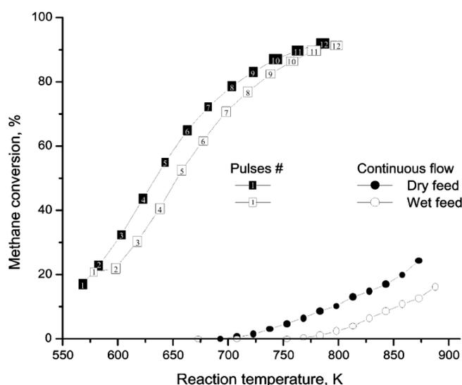
**Figure 3.** Temperature-programmed reactions during pulsed or continuous flow of reactants over Pd/ZrO<sub>2</sub> with or without H<sub>2</sub>O in the feed. Reproduced with permission from [42]. Copyright © 2001 Elsevier.
