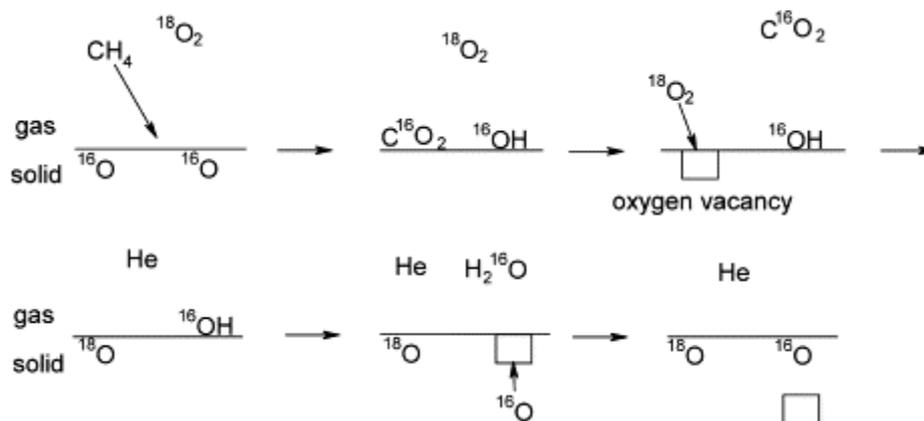
**Figure 13.** Schematic of oxygen exchange during CH<sub>4</sub> oxidation using labeled pulsed experiments. Reproduced with permission from [70]. Copyright © 2002 Elsevier.
