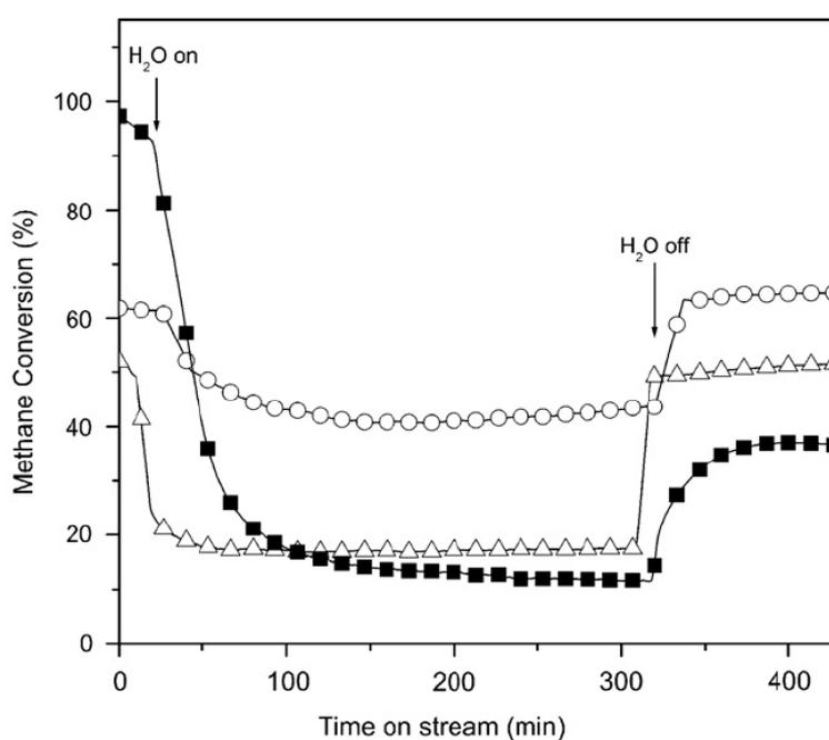
**Figure 1.** Effect of water vapor on the activity for CH<sub>4</sub> combustion over Pd/Al<sub>2</sub>O<sub>3</sub> (■); 2:1 PdPt/Al<sub>2</sub>O<sub>3</sub> (Δ); and 1:1 PdPt/Al<sub>2</sub>O<sub>3</sub> (○) at 500 °C; 5 vol.% of steam was added to the 1.5% CH<sub>4</sub>/air feed gas, GHSV = 100,000 h<sup>-1</sup>, for 5 h. [35] Copyright© 2007 Elsevier.
