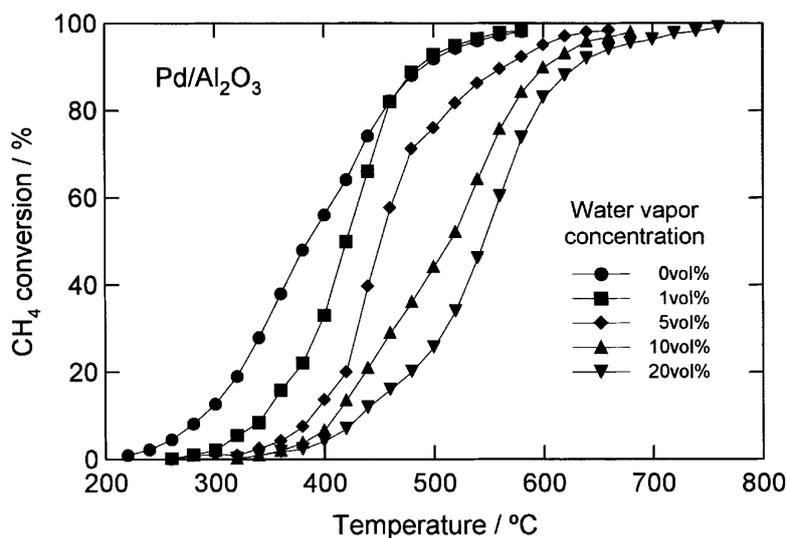
**Figure 6.** Catalytic combustion of CH<sub>4</sub> over 1.1 wt.% Pd/Al<sub>2</sub>O<sub>3</sub> with different amounts of water added (vol.%). Reaction conditions: CH<sub>4</sub>, 1 vol.%; O<sub>2</sub>, 20 vol.%; H<sub>2</sub>O, 0–20 vol.%; N<sub>2</sub>, balance; GHSV 48,000 h<sup>-1</sup>. Reprinted with permission from [16]. Copyright © 2002 Elsevier.
