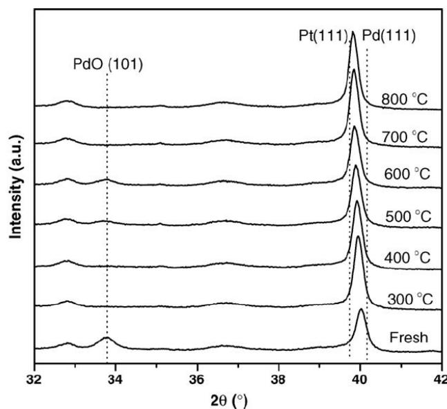
**Figure 14.** High-temperature *in situ* XRD profiles of PdPt-Al<sub>2</sub>O<sub>3</sub> during heating. Reprinted with permission from [64]. Copyright © 2006 Elsevier.
