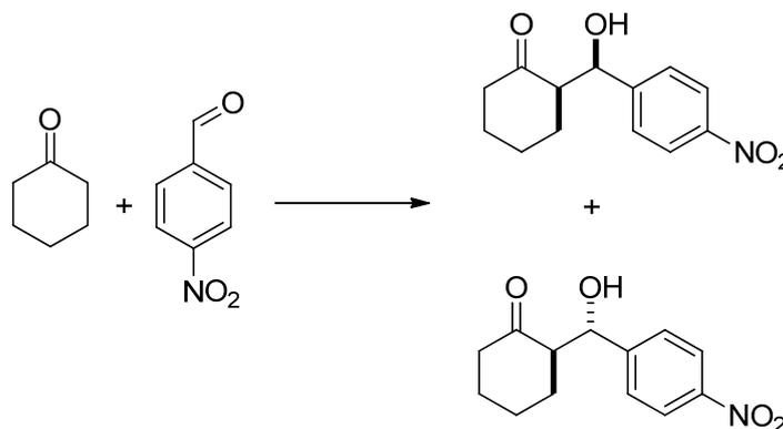
**Table 1.** Aldol reaction with cyclohexanone (20 equiv.), 4-nitrobenzaldehyde (1 equiv.) and chitosan (*ca.* 100 mg  $\approx$  2 equiv. primary amine functions) dissolved in different ionic liquids (1 g) and different additives (20 mol%) for 4 days at 37 °C.
