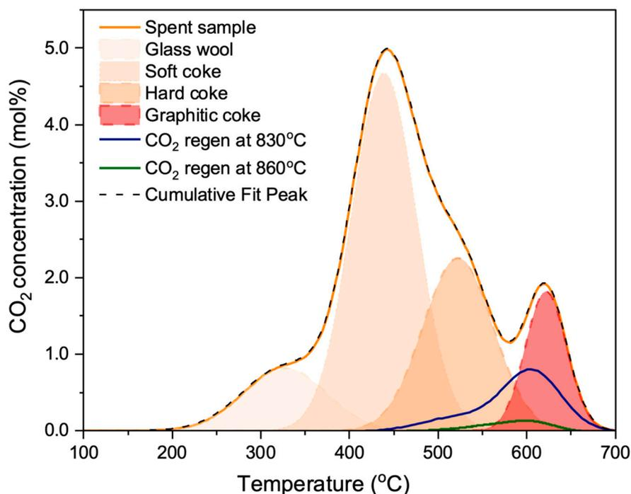
**Figure 9.** Temperature-programmed oxidation (TPO) on a spent coked sample (deactivated via MDA reaction at 700 °C for 14 h at WHSV of 936 cc/g/h in 50%CH<sub>4</sub> in Ar flow), a CO<sub>2</sub>-regenerated spent sample at 830 °C for 30 min, and a CO<sub>2</sub>-regenerated spent sample at 860 °C for 30 min. TPO analysis revealed that CO<sub>2</sub> preferentially removes soft coke, while hard coke persists until 830 °C.
