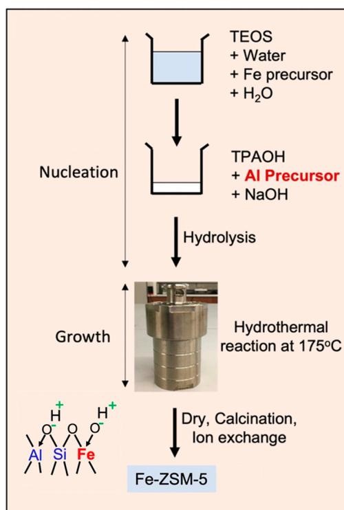
**Figure 1.** Synthesis procedure for isomorphously substituted Fe-ZSM-5 catalyst.
