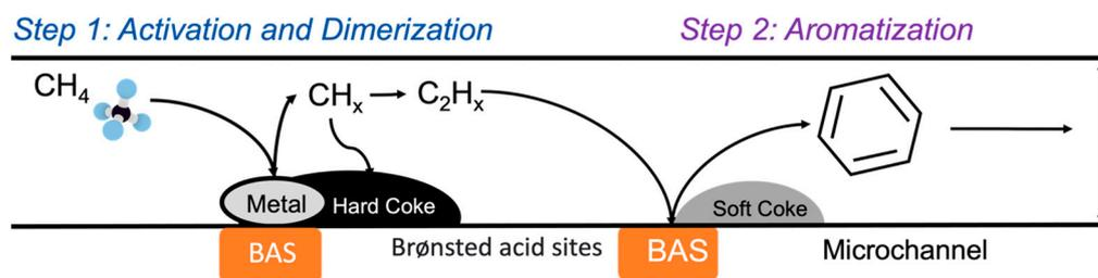
**Figure 8.** Schematic illustrating the formation of different types of coke (soft versus hard coke) on active sites.
