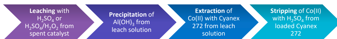
Figure 1. Four-step process for hydrometallurgical recovery of Co(II) from CoMo catalyst of hydrodesulfurization.
