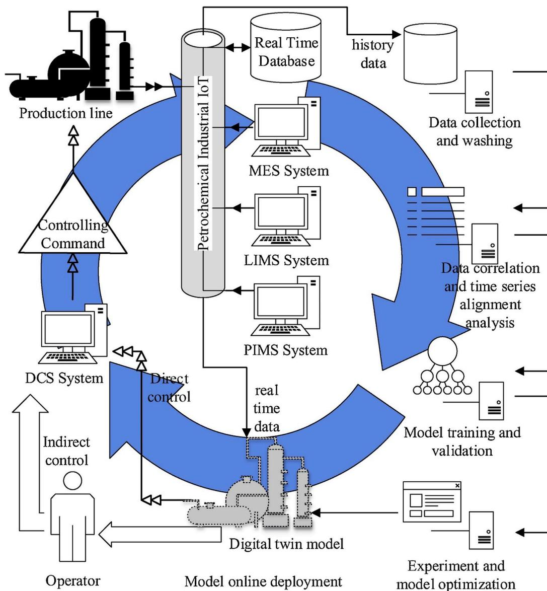
**Figure 6.** Digital twin practice loop using machine learning techniques. Reused with permission from Min et al. [10].
