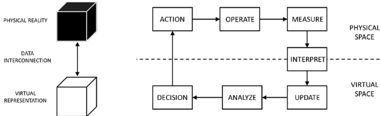
**Figure 3.** Components and high-level processes of Digital Twin. Reused with permission from VanDerHorn and Mahadevan [26].
