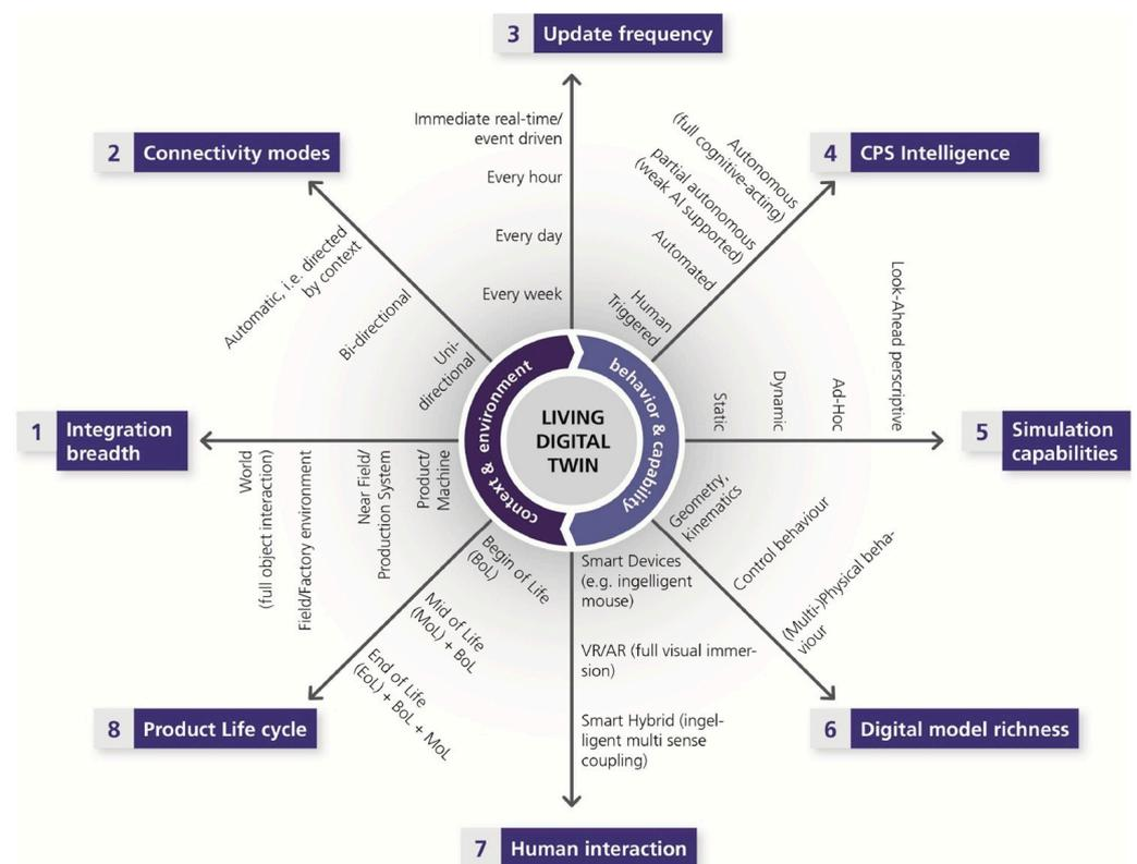
**Figure 7.** The Digital Twin 8-D model. Reused with permission from Stark et al. [50].
