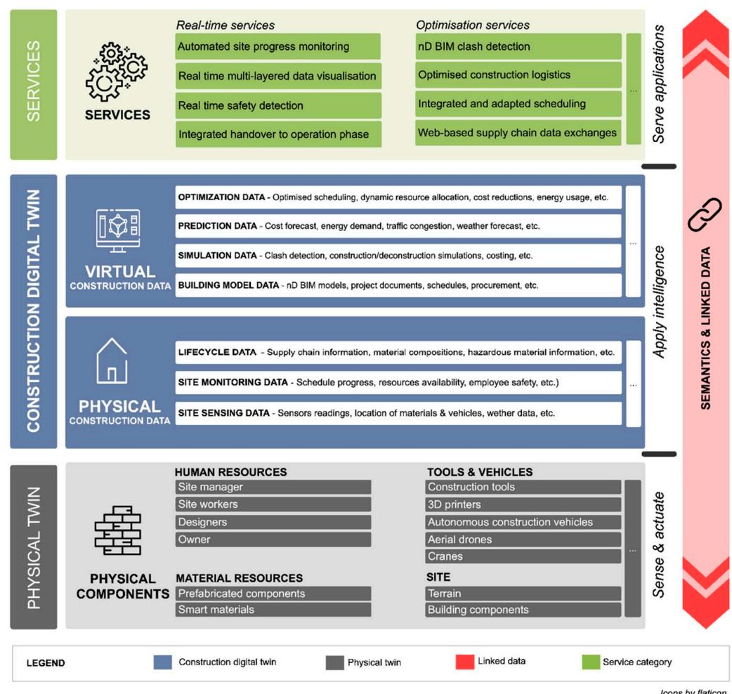
Figure 9. Utilization of construction Digital Twin data for enabling smart construction services. Reused with permission from Boje et al. [60].
