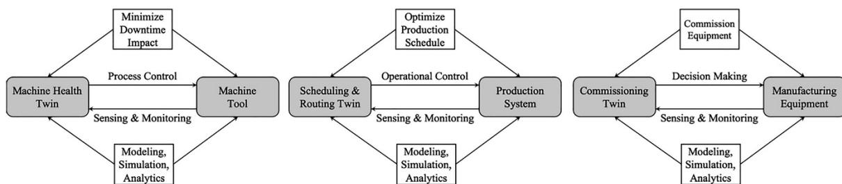
**Figure 5.** Three instances of digital twin utilization in manufacturing processes. Reused with permission from Shao and Helu [31].
