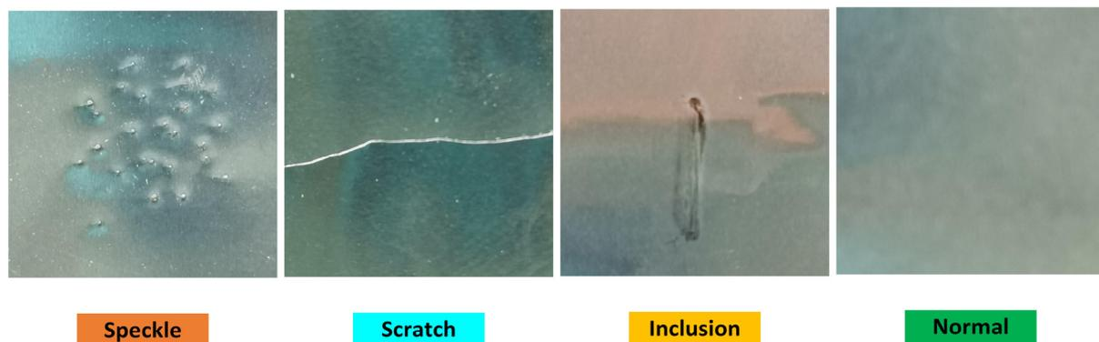
**Figure 1.** Defect images surface: defects and normal workpieces.
