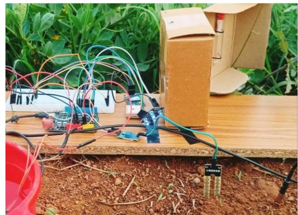
**(b)** Sensor connectivity using Arduino**Figure 2.** Cont.
