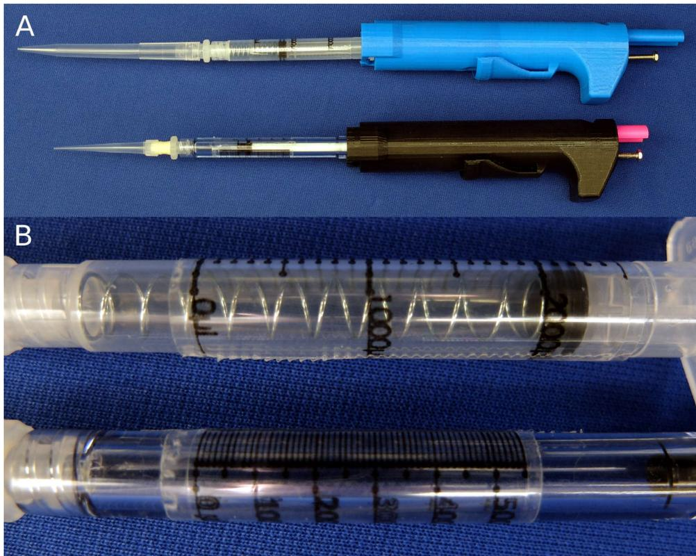
**Figure 4.** Photos of assembled pipettes. (A) Two assemblies of the pipette: the 100–1000- $\mu\text{L}$  configuration (top) and the 30–300- $\mu\text{L}$  configuration (bottom). (B) Close-up photo of the taped on scale for each of the syringes. Scales are available in the Appendix A: Figures A1 and A2.
