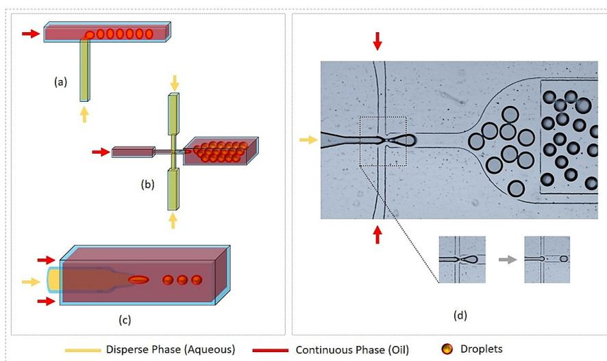
**Figure 1.** Droplet generation by microfluidic systems. (a) T-junction; (b) Flow-focusing; (c) Co-flow (glass capillary); (d) Droplet generation by flow focusing device (use of fluorinated oil with stabilizing agent and disperse phase as water solution of dye), device also includes on-chip storage pool for droplet collection and operation region.
