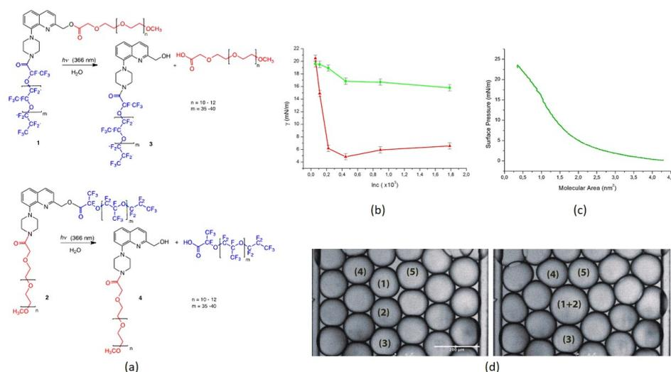
**Figure 7.** Surfactants 1 and 2: (a) Chemical composition; (b) Interfacial tension versus concentration, red curve for Surfactant 1 and green curve for Surfactant 2; (c) Surface pressure versus molecular area; (d) Light-induced merging of droplets 1 and 2. Reproduced with permission from [32].
