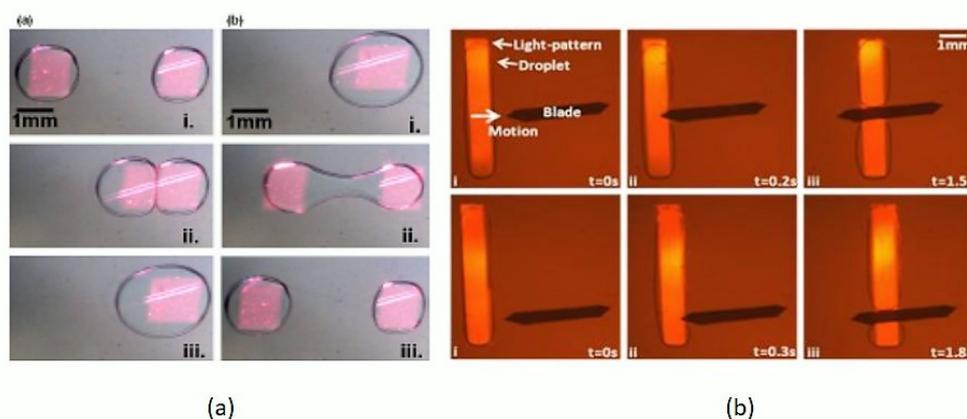
**Figure 6.** Optical droplets merging and sorting: (a) Square-shaped projection patterns moving two droplets towards each other, merged, and sliced back to acquire two droplets. Reproduced with permission from [135]; (b) Time sequences of an elongated droplet sliced by on-chip Teflon blade, droplet motion assisted by line projection. Reproduced with permission from [136].
