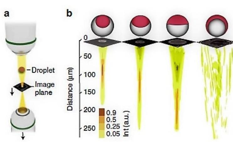
**Figure 8.** Imaging using microdroplets: setup for light input from the top with an adjustable image plane, droplets on a substrate, image plane, and bottom collection objective with vertical translation, characteristic focal length tunability based on the morphology of the emulsion, and corresponding fully converging-to-fully diverging mechanism. Reproduced with permission from [63].
