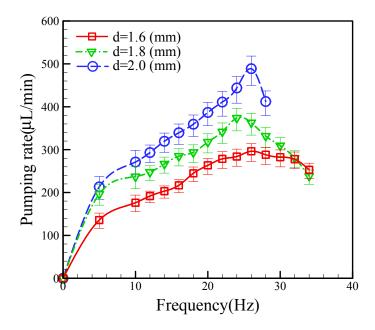
**Figure 6.** Relationship between pumping rate and different locations of the active check valve as a function of operational frequency at a pneumatic pressure of 68.9 kPa.
