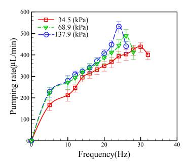
**Figure 7.** Relationship between the pumping rate and pneumatic pressures at different operating frequencies.
