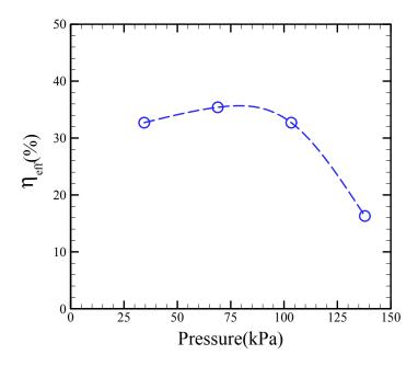
Figure 8. Pumping efficiency of the proposed micropump against applied pressure.
