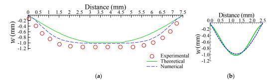
**Figure 4.** Theoretical, numerical, and experimental results for the (**a**) x-directional and (**b**) y-directional deformations at a pneumatic pressure of 68.9 kPa.
