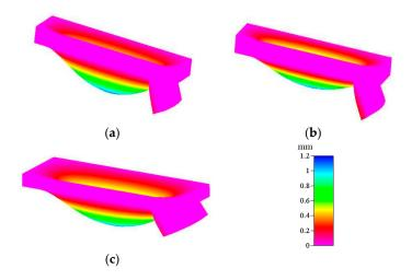
**Figure 5.** Deflections of the actuated membrane with the active check valve at different locations: (a) 1.6 mm; (b) 1.8 mm, and (c) 2.0 mm at a pneumatic pressure of 68.9 kPa.
