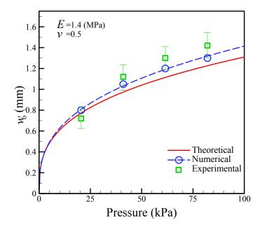
**Figure 3.** Comparison of maximum deformations between theoretical calculations, numerical simulations, and experimental measurements at different air pressures.
