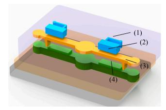
**Figure 1.** Schematic illustration of the proposed micropump. (1), (2), (3), and (4) indicate the air chamber, actuated membrane, active check valve, and bottom-protruding structure, respectively.
