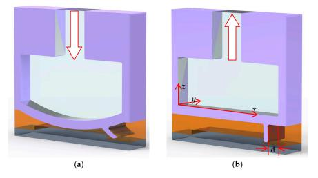
**Figure 2.** Schematic illustration of the actuation mechanism of the micropump. (a) The actuated membrane is activated by an active check valve to generate forward flow. (b) The active check valve is blocked by the bottom-protruding structure to prevent backflow. Red arrows indicate air flow in/out.
