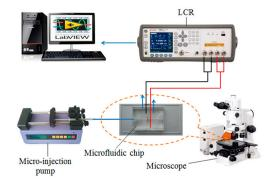
Figure 5. Schematic diagram of impedance detection system.
