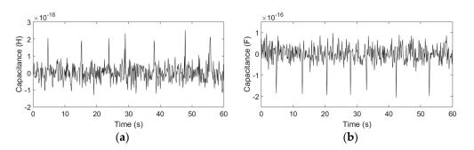
**Figure 11.** Detection results of water droplets and bubbles, the frequency was 0.3 MHz and each coil had 20 turns: (**a**) water droplets with sizes ranging from 100 to 110  $\mu$ m; (**b**) bubbles with sizes ranging from 180 to 200  $\mu$ m.
