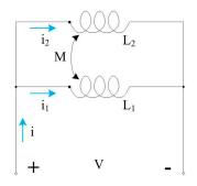
**Figure 2.** Schematic diagram of inductance detection:  $L_1$  and  $L_2$  are single-layer coil 1 and single-layer coil 2, respectively.  $i_1$  and  $i_2$  are the alternating currents that flow through the two coils.
