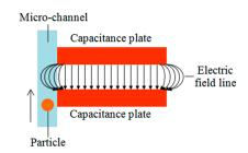
Figure 4. Electric field distribution of parallel plate capacitor.
