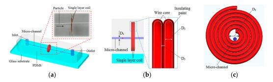
**Figure 1.** The design of the on-chip impedance sensor: (a) The overall design of the chip; (b) cross-section of the chip:  $D_1$  is the diameter of the micro-channel,  $D_2$  is the diameter of the coil wire core,  $D_3$  is the distance between the two single-layer coils; (c) a sketch of a single-layer coil:  $D_4$  is the inner diameter of the single-layer coil.
