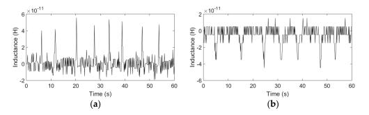
**Figure 8.** Detection results of iron and copper particles, the frequency was 2 MHz and each coil had 20 turns: (**a**) iron particles with sizes ranging from 40 to 50  $\mu$ m; (**b**) copper particles with sizes ranging from 110 to 120  $\mu$ m.
