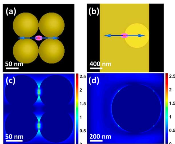
**Figure S1.** Representative (a) OS and (b) SM architectures. Calculated E-field distribution for (c) OS and (d) SM architectures. The incident wavelength is 785 nm.
