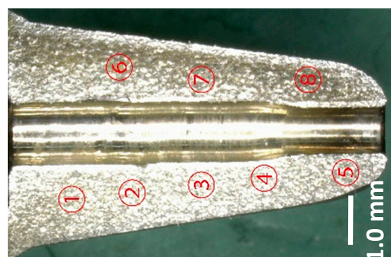
Figure 6. Outlet of mini-nozzle after plasma nitriding at 693 K for 14.4 ks.
