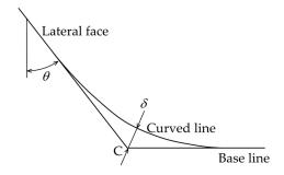
**Figure 13.** The forming accuracy based on distance  $\delta$  from point C to the pyramid profile.
