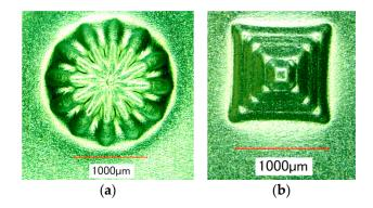
**Figure 11.** Other pyramids formed by ultrasonic incremental microforming: (**a**) pyramid like sunflower; (**b**) stepwise pyramid.
