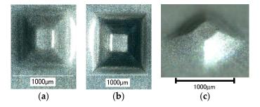
**Figure 14.** Titanium pyramids of D = 1.41 mm formed with ultrasonic vibration: (**a**) top view; (**b**) bottom view; (**c**) high angle view.
