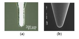
**Figure 3.** Microtool for incremental microforming: (a)  $R = 100 \mu m$ ; (b)  $R = 10 \mu m$ .
