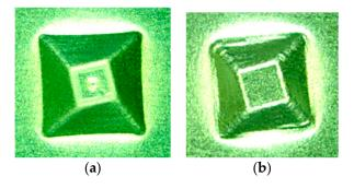
**Figure 8.** Top views of twisted pyramids formed: (**a**) with ultrasonic vibration; (**b**) without ultrasonic vibration.
