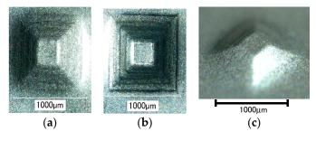
**Figure 15.** Titanium pyramids of D = 1.41 mm formed without ultrasonic vibration: (**a**) top view; (**b**) bottom view; (**c**) high angle view.
