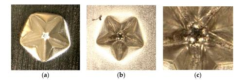
**Figure 10.** Top and bottom views of a star pyramid formed without ultrasonic vibration: (**a**) top view; (**b**) bottom view; (**c**) magnified center part of bottom view.
