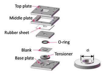
Figure 2. Blank holder and tensioner.
