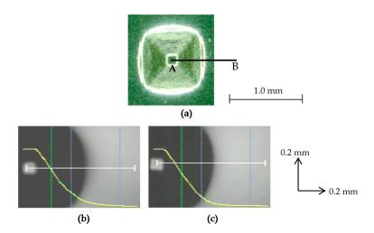
**Figure 12.** Profiles of pyramids of stainless steel foil under different conditions: (**a**) top view of a pyramid formed without ultrasonic vibration and heating; (**b**) surface profile along AB in the case of NV and NH; (**c**) surface profile along AB in the case of V and H.
