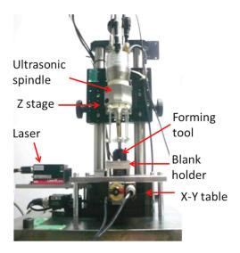
Figure 1. Desktop microforming machine.
