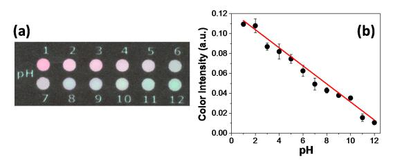
**Figure 2.** Presentation of (**a**) an optical micrograph showing the color changes on printed zones and (**b**) color intensity analysis over different pH values. In (a), microzones were first spotted with 5  $\mu$ L of the natural indicator. Then, 5  $\mu$ L of different solutions prepared at pH range from 1 to 12 were added on microzones prior to image capture. The labels depicted in (a) indicate the used microzones for each pH value.
