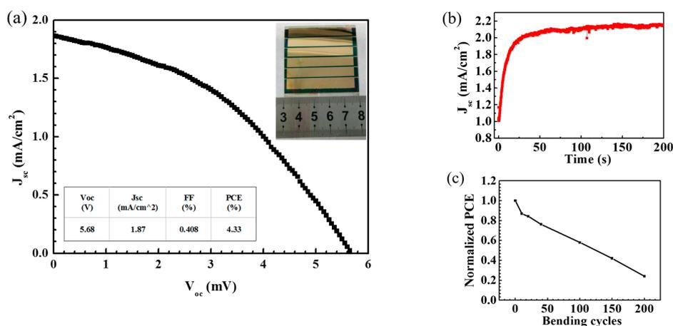
**Figure 9.** (a) J-V characteristics of a typical flexible PSC of 5 cm × 5 cm with an active area of 13.5 cm<sup>2</sup>, tested without a mask. Inset photograph is the typical flexible PSC. (b) Photocurrent density measured as a function of time for the same flexible PSC held at 2.5 V forward bias. (c) Normalized PCE of the large-area flexible PSC after bending tests using 50 mm radii of curvature.
