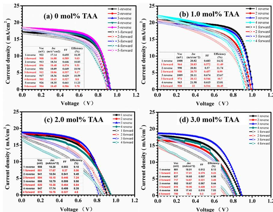
**Figure 5.** J-V characteristics of the gas-assisted processed PSCs based on TiO<sub>2</sub> compact layer deposited by the ultrasonic spray-coating of TiO<sub>2</sub> solution with the addition of TAA (a) 0 mol %; (b) 1.0 mol %; (c) 2.0 mol %; (d) 3.0 mol % with respect to the TiO<sub>2</sub> content.
