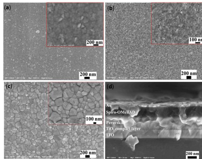
**Figure 4.** Scanning electron microscopy (SEM) image of (a) PEN-ITO substrate; (b) TiO<sub>2</sub> compact layer; (c) perovskite prepared by the gas-assisted method; and (d) cross-section SEM image of the PSCs.
