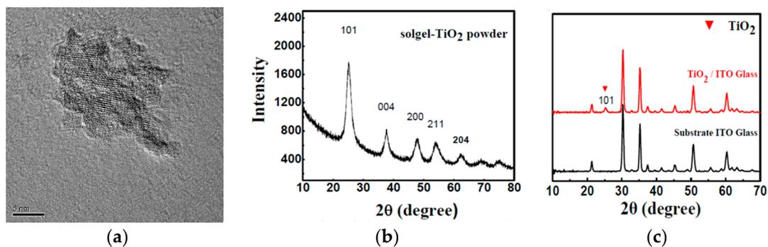
**Figure 2.** (a) Transmission electron microscopy (TEM) image of the TiO<sub>2</sub> nanoparticles dispersed in ethanol at a concentration of 1.0 mg/mL; (b) XRD pattern of the TiO<sub>2</sub> powder drying at 135 °C; and (c) XRD patterns of ITO-glass with/without the TiO<sub>2</sub> compact layer coated by the ultrasonic spraying.
