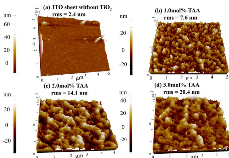
**Figure 6.** AFM images of the surface of the  $\text{TiO}_2$  layers sprayed by the  $\text{TiO}_2$  ethanol solution with the addition of TAA, (a) ITO sheet without  $\text{TiO}_2$  film; (b) 1.0 mol % TAA; (c) 2.0 mol % TAA; and (d) 3.0 mol % TAA with respect to the  $\text{TiO}_2$  content.
