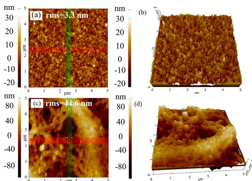
**Figure 3.** Atomic force microscope (AFM) images of the surface of the TiO<sub>2</sub> layers sprayed by (a,b) the w-film; (c,d) the d-film using the TiO<sub>2</sub> ethanol solution without TAA.
