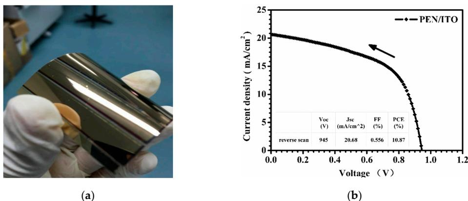
**Figure 8.** (a) Photographic image of the flexible device with a large area of 5.0 cm × 5.0 cm and (b) J-V curve of the flexible device fabricated by using the optimized parameters of ultrasonic spraying on polymer ITO-PEN substrate, tested under AM 1.5 G sunlight (100 mW/cm<sup>2</sup>) using a metal mask of 0.16 cm<sup>2</sup>.
