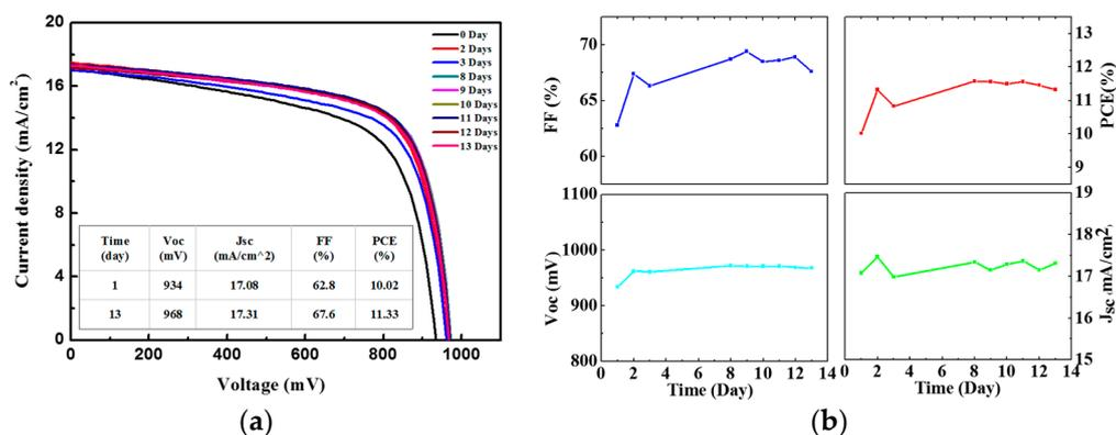
**Figure 7.** Long-duration stability test of a typical PSC based on ITO-glass, measured under AM 1.5 G sunlight (100 mW/cm<sup>2</sup>) using a metal mask of 0.16 cm<sup>2</sup>. (a) J-V curve of the PSC; and (b) FF, PCE, J<sub>sc</sub>, V<sub>oc</sub>.
