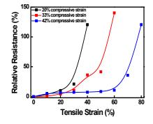
Figure 4. Resistance changes of wrinkled hybrid electrodes according to mechanical tensile strains.
