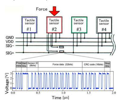
Figure 12. Packet communication for the tactile sensor network.
