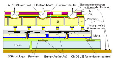
Figure 17. Schematic of a Pierce-type nc-Si electron emitter array stacked with a driving LSI.
