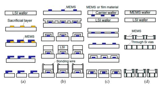
**Figure 1.** Heterogeneous integration processes; (**a**) surface micromachining; (**b**) assembly of packaged MEMS and LSI; (**c**) wafer-level transfer of MEMS to LSI (combined with a wafer level packaging); and (**d**) stacked integration using through Si vias.
