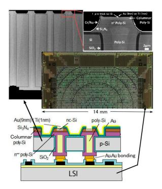
Figure 14. Structure of planer-type active matrix electron source using the nc-Si electron emitter.
