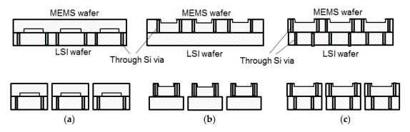
**Figure 9.** Stacked integration using through Si vias (TSVs); (**a**) LSI wafer vias; (**b**) MEMS wafer vias; and (**c**) LSI wafer vias and MEMS wafer vias.
