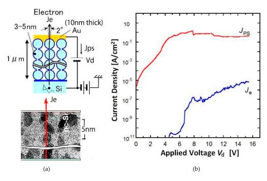
Figure 13. nc-Si electron emitter; (a) principle; and (b) characteristics.
