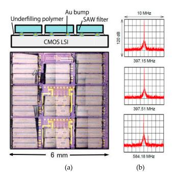
**Figure 8.** Multi SAW resonators on a LSI chip; (**a**) structure and photograph; and (**b**) frequency spectrums of three SAW oscillators on LSI.
