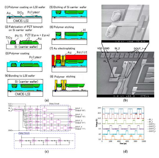
**Figure 5.** PZT MEMS switch on LSI; (**a**) fabrication process; (**b**) photographs; (**c**) circuit; and (**d**) waveform from the circuit.
