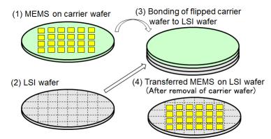
Figure 2. Concept of the heterogeneous integration by the wafer-level transfer.
