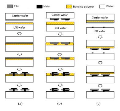
**Figure 3.** Wafer level transfer of heterogeneous MEMS to LSI; (**a**) film transfer; (**b**) device transfer connectivity last; and (**c**) immediate connectivity at device transfer.
