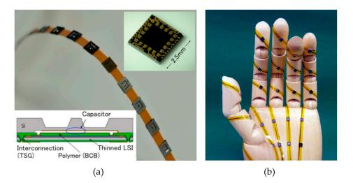
Figure 10. Tactile sensor network; (a) structure and photograph; and (b) application.
