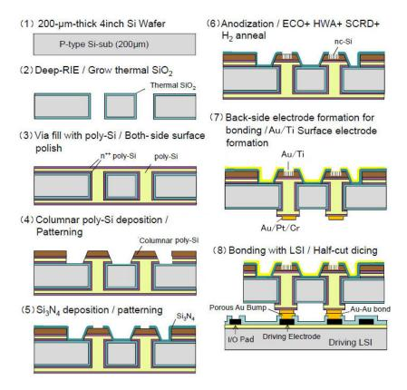
Figure 15. Fabrication process of planer-type active matrix electron source.
