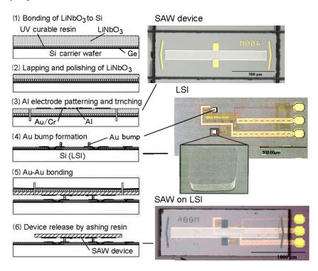
Figure 6. Fabrication process of SAW resonator on LSI.
