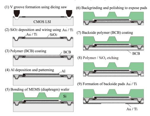
Figure 11. Fabrication process of the tactile force sensor on LSI.
