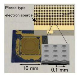
Figure 18. Photographs of Pierce-type nc-Si electron emitter array.
