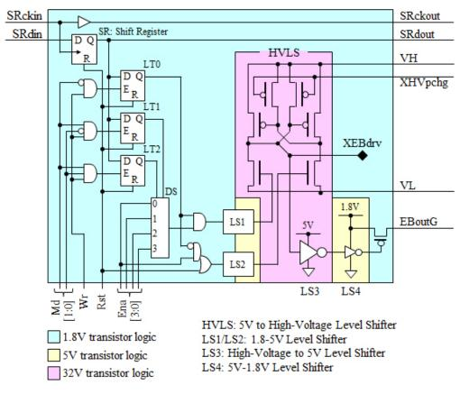
**Figure 16.** Circuit of one cell in the  $100 \times 100$  active matrix driving LSI.
