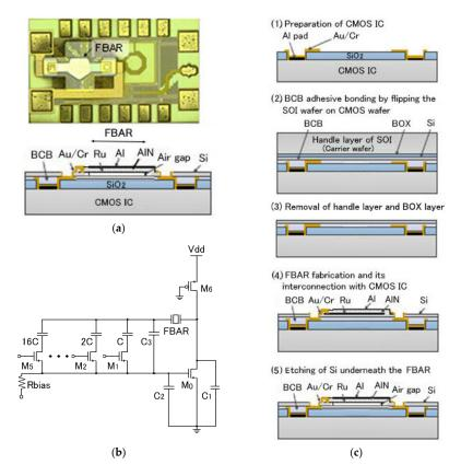
**Figure 4.** FBAR on LSI; (**a**) photograph and structure; (**b**) CMOS oscillation circuit; and (**c**) fabrication process.
