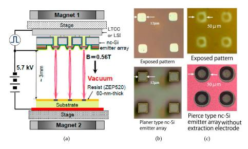
Figure 19. 1:1 electron beam exposure; (a) exposure system; (b) planer type; and (c) Pierce type.
