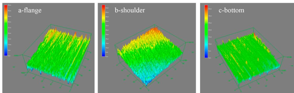
**Figure 11.** The 3D plot of surface roughness when the laser energy was 1550 mJ.
