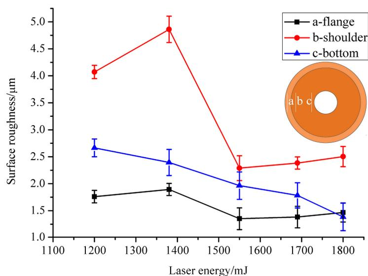
**Figure 10.** The relationship between the laser energy and the surface roughness value on three different areas.
