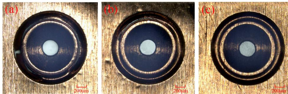
**Figure 8.** The morphology of the work piece under the laser energy of 1550 mJ when the thickness of the soft punch is (a) 200 μm (b) 300 μm (c) 400 μm.
