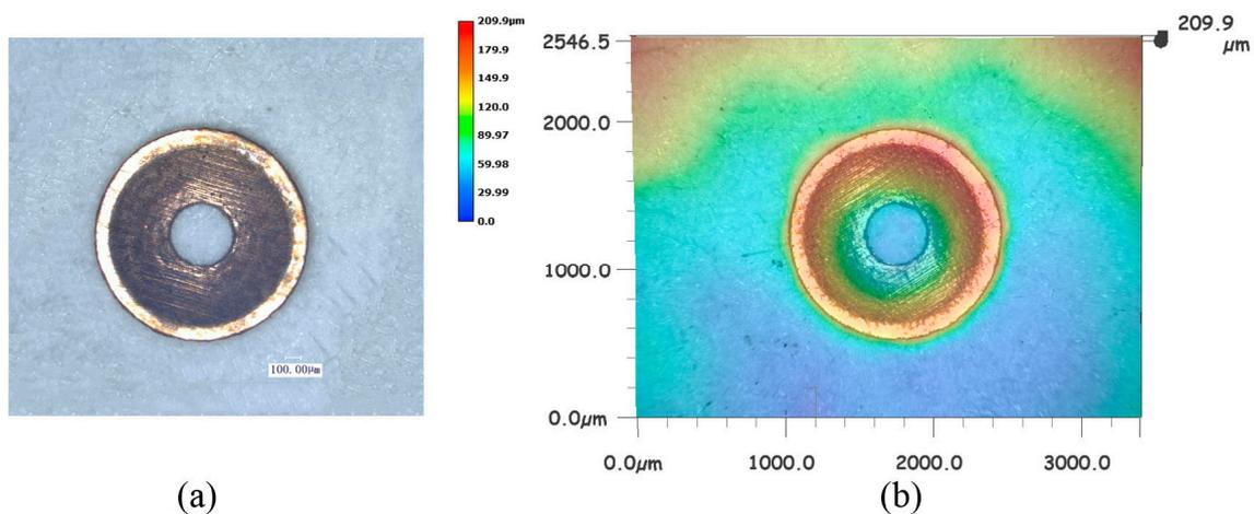
**Figure 5.** The morphology of a micro-part when a laser energy of 1550 mJ was employed on the work piece: (a) 2D plot of the dish-shaped micro-part; (b) 3D plot of the dish-shaped micro-part.
