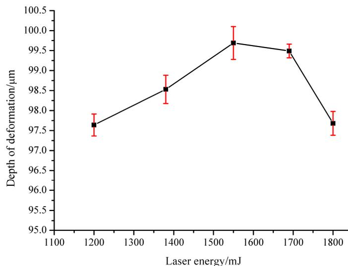
**Figure 6.** The relationship between the laser energy and deformation depth when the thickness of soft punches was 200  $\mu\text{m}$ .
