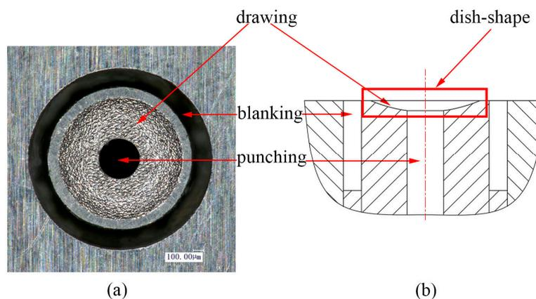
**Figure 3.** (a) Two-dimensional plot of the compound die; (b) cross-section of the compound die.
