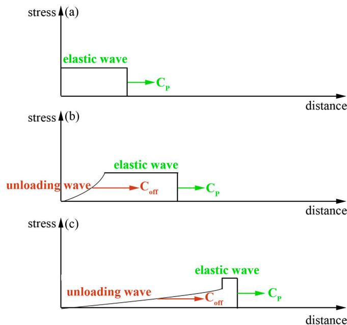
**Figure 9.** Schematic propagation of elastic waves:  $C_p$  is the velocity of the elastic wave;  $C_{off}$  is the velocity of the unloading wave. (a) Only elastic wave; (b) unloading wave occurs; (c) the elastic wave is almost be caught up by unloading wave.
