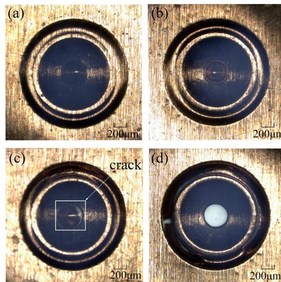
**Figure 4.** Two-dimensional plot of the work piece when the laser energy is (a) 565 mJ; (b) 675 mJ; (c) 835 mJ; (d) 1200 mJ.
