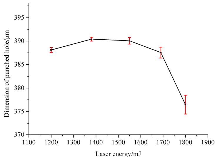
**Figure 7.** The relationship between laser energy and the dimension of the punched hole.
