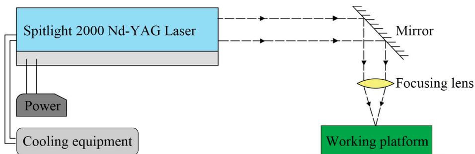
Figure 1. Schematic of the laser machining equipment.
