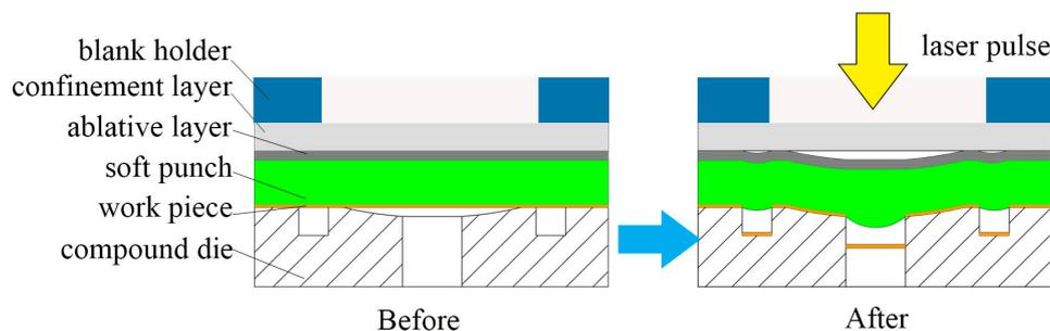
Figure 2. Schematic of the working platform and laser compound process.
