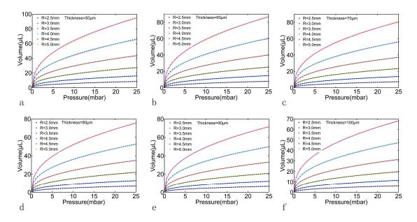
**Figure 6.** The pressure-volumes relationships of the PDMS membrane with different radius *R* and different thickness *h* derived from the FEM analysis. Subplot (a-f) represent the thickness of the PDMS membrane from 50 to 100 µm with 10 µm a step.
