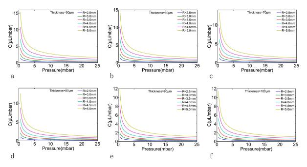
**Figure 7.** The pressure-capacitance relationships of the PDMS membrane with different radius *R* and different thickness *h* derived from the FEM analysis and Equation (8). Subplot ( $\mathbf{a}$ - $\mathbf{f}$ ) represent the thickness of the PDMS membrane from 50 to 100 µm with 10 µm a step.
