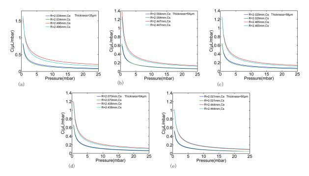
**Figure 11.** The experimental pressure-capacitance relationship of the PDMS membrane. "Ce" and "Cs" are the hydraulic capacitances obtained by experiments and theoretical estimation respectively. Subplot (**a–e**) represent the thickness of the PDMS membrane from 35 to 90  $\mu$ m.
