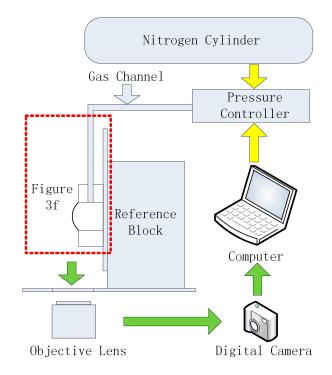
**Figure 4.** The experimental setup for PDMS membrane testing. The nitrogen bottle acted as a source of the gas pressure, the pressure controller accepted orders from the computer to control its output pressure and connected with the testing device in Figure 3 by gas channel, the testing device was fixed on the reference block to keep vertical to the stage, the digital camera captured the images of the deflected membrane through the objective lens.
