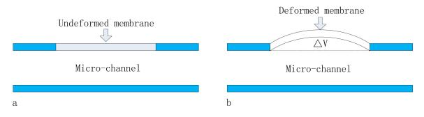
**Figure 1.** The cross section of a membrane-based microfluidic capacitor: (**a**) an uncharged capacitor and (**b**) a charged capacitor.
