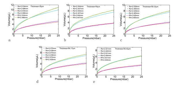
**Figure 10.** The experimental pressure-volume relationships of the PDMS membrane with different radius *R* and different thickness *h*. The "Re" dot plot indicate the results of the experiments and the "Rf" solid lines indicate the results of fitting the experimental data. The "Rs" solid line indicate the theoretical estimation using the same geometry parameters and Equations (13)–(15). Subplot (**a**–**e**) represent the measured thickness of the PDMS membrane from 35 to 90  $\mu$ m.
