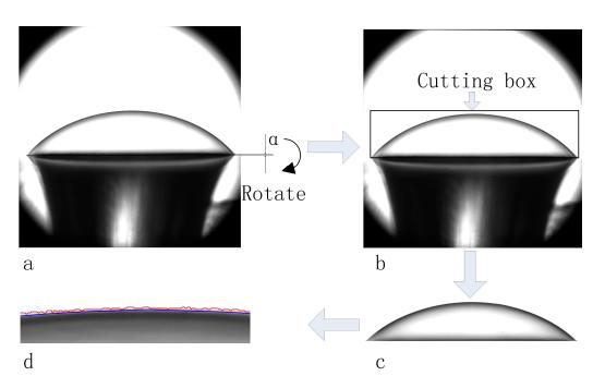
**Figure 5.** Flow chart for the proposed image processing method to obtain the outer boundary of the deformed membrane: (**a**) the original image with an image rotation angle  $\alpha$ ; (**b**) the result of rotating and cutting the image using a region of interest (ROI) box; (**c**) the result of cutting; (**d**) the result of segmentation by thresholding method (red line) and the level set method (blue line).
