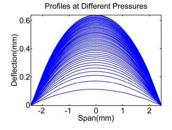
**Figure 9.** Profiles of deformed membrane in experiments, the exerted pressures are from 0 to 25 mbar with the step of 0.5 mbar.
