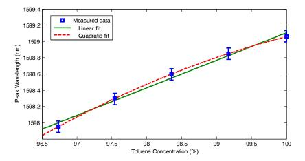
**Figure 11.** The position of the maxima wavelength *versus* the toluene concentration in the toluene-acetone mixture.
