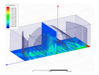
**Figure 7.** The electric field distribution of higher order resonance mode at 1542 nm for the test liquid  $n_t = 1.3$ .
