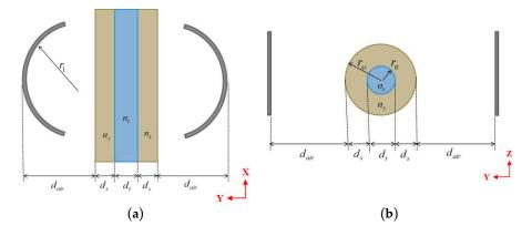
**Figure 3.** Schematic diagram for: (a) the horizontal cross section and (b) the vertical cross section, of the cylindrical Fabry-Pérot cavity with the micro tube inside indicating the design parameters and geometry.
