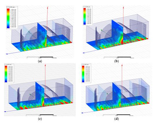
**Figure 6.** The electric field distribution at resonance for different test liquids (**a**)  $n_t = 1.18$ , resonance at 1528 nm; (**b**)  $n_t = 1.3$ , resonance at 1576 nm; (**c**)  $n_t = 1.6$ , resonance at 1511 nm; (**d**)  $n_t = 1.8$ , resonance at 1505.7 nm.
