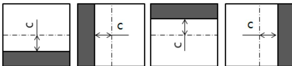
Figure 10. Definition of clearance gap  $c$ .
