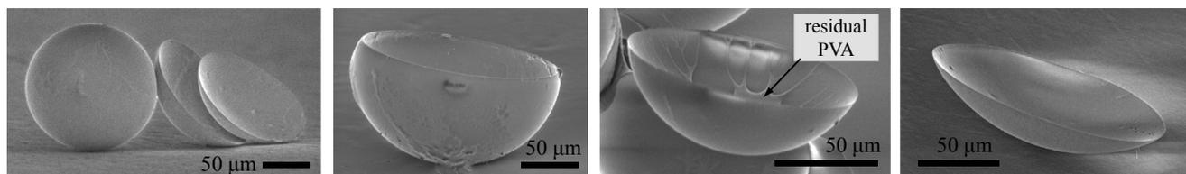
**Figure 8.** Various shapes of capsules, bowl-like and lens-like, resulting from different solidification conditions.
