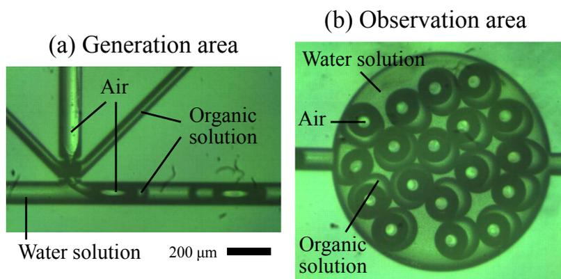
**Figure 3.** Images of G/O/W microdroplets in (a) the generation area within the multiphase junction and (b) the observation area.
