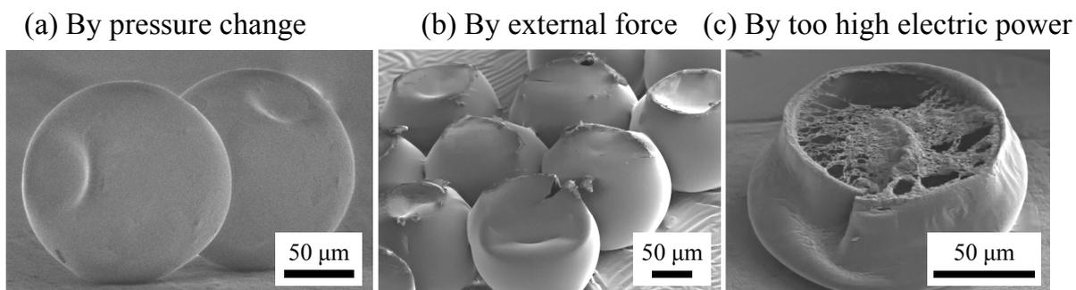
**Figure 7.** Images of deformed capsules: (a) By pressure change; (b) by external force; (c) by too high electric power.
