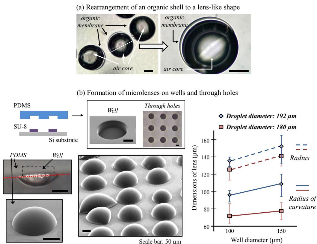
**Figure 9.** (a) Rearrangement of organic shell layers; (b) on-demand microlens formation on a polydimethylsiloxane (PDMS) structure.
