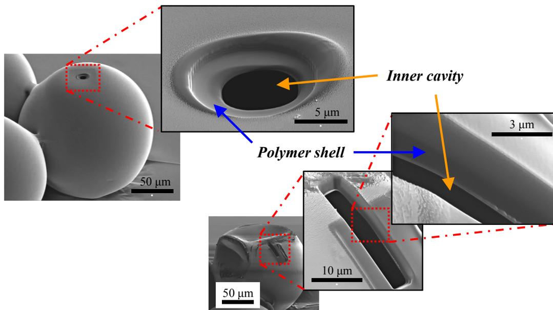
**Figure 6.** Partially etched microcapsules using focused ion beam (FIB) lithography showing shell membranes and inner cavities.
