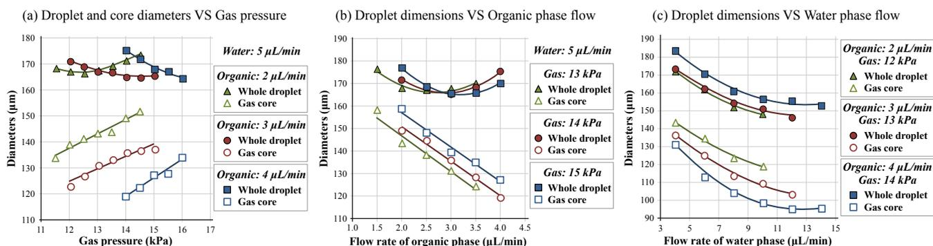
**Figure 4.** Results of the multiphase droplet generation that occurred by controlling the flow rate of each phase fluid. (a) Droplet and core diameters vs. gas pressure; (b) droplet dimensions vs. organic phase flow; (c) droplet dimensions vs. water phase flow.
