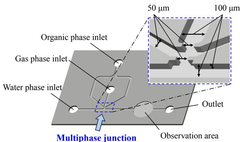
**Figure 2.** Silicon wafer design for microdroplet generation and, in the inset, detail of the multiphase junction.
