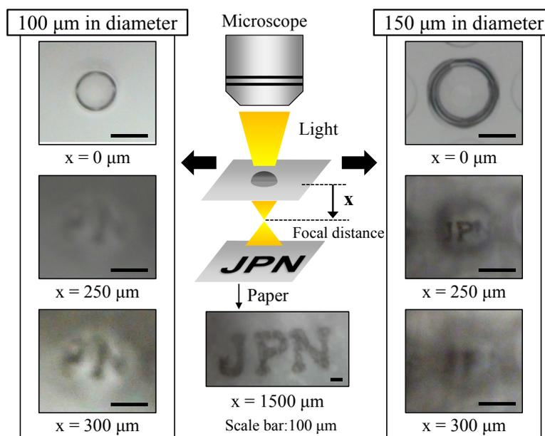
**Figure 10.** Optical microscope images of different microlenses formed by the same droplets but on different wells.
