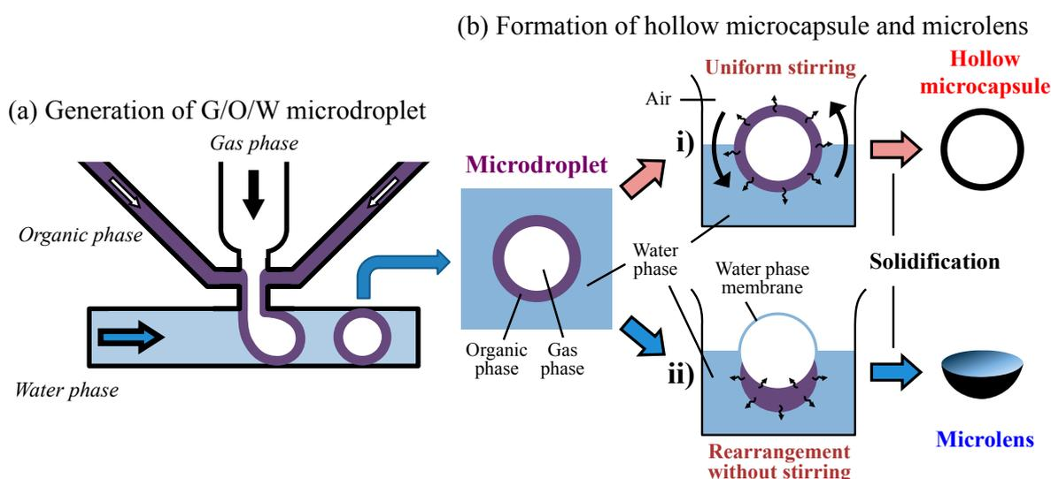
**Figure 1.** Steps in the formation of microcapsules and microlenses using gas-in-organic-in-water (G/O/W) microdroplets. (a) Generation of G/O/W microdroplet; (b) formation of hollow microcapsule and microlens.
