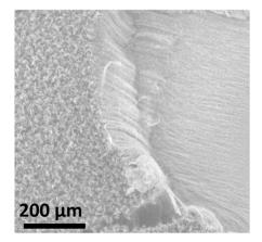
The pattern repeatability and accuracy of the laser-etching post-process can be controlled through the etching parameters and is dependent on the quality of the CNT brush-growing process (flatness/rugosity of the quartz substrate and adhesion strength of the CNT onto its surface). The resulting pattern is observed to be reproducible. The wavelength of the laser pulse is 355 nm. The spot diameter in the focal plane is close to 10  $\mu$ m.
