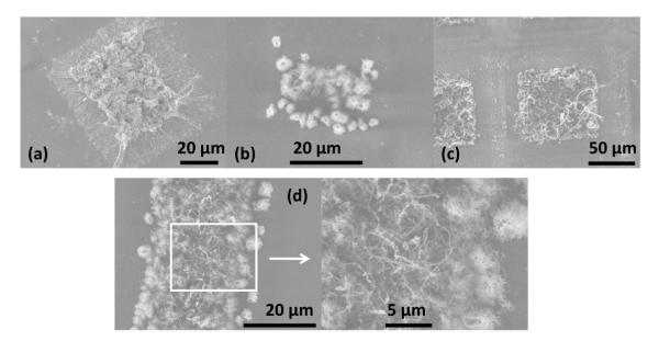
The quality and the resolution of the pattern depend on the height of the CNT and limitations of our laser process. The height of the CNT array is fixed by the CVD process parameters. The power must be decreased when the CNT length is less than 50  $\mu$ m in order to preserve the CNT structure. In the focus plane, the lowest etched surface has a diameter of 10  $\mu$ m, and the final structures can have a minimal resolution of 10  $\mu$ m, with a minimal period of 50  $\mu$ m.
