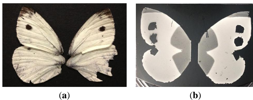
Figure 6. (a) Actual Pieris rapae butterfly wings showing white coloration with black spots; (b) result of Pieris rapae replication: the white surface is produced by SU-8 beads with diameters in the range of 100 to 500 nm. Black dots are the result of the black pyrolyzed layer without beads.
