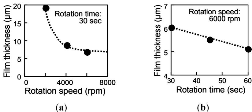
It was found that the film thickness became nonuniform when the rotation time largely exceeds 30 s, as shown in Figure 5. This result indicates that a smooth polyurethane film which is thinner than about 6  $\mu\text{m}$  cannot be formed only by the spin-coating method.
