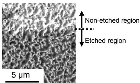
Figure 7. Decrease of film thickness by etching-back using sulfuric acid.
