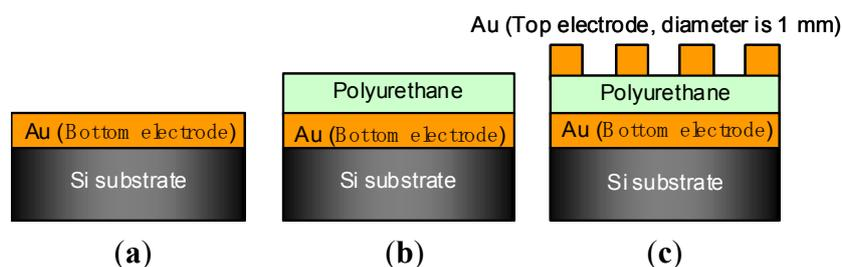
Figure 9. Photograph of fabricated tactile sensors using poly-urethane thin film and Au electrodes. Diameter of circular Au electrode (dark gold color) is 1 mm.
