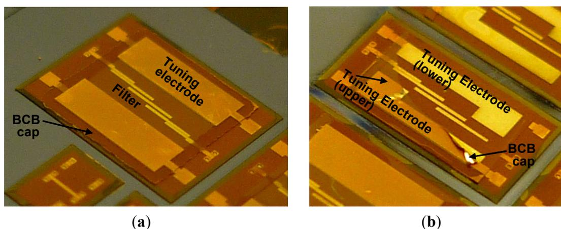
In general, BCB cap has downward deflection due to its tensile residual stress as presented in [9]. As a reference, a BCB cap profile without gold electrode is given in Figure 7(b). The BCB cap profile of the fabricated tunable filter is investigated because it determines the behaviour of the BCB cap actuation. As shown in Figure 7, the BCB membrane has  $5\ \mu\text{m}$  upward deflections at its center due to the residual stress effect between BCB cap and upper gold electrodes.
