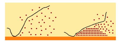
**Figure 9.** Schematic diagram of nanoparticle deposition in microlayer evaporation during boiling. Nanotubes
