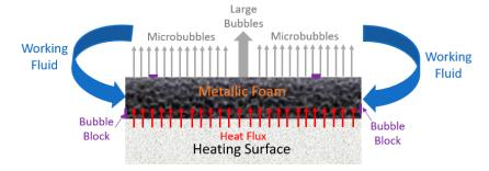
**Figure 20.** Schematic illustration of the nucleate boiling mechanism using a metallic foam attachment. Adapted from [152].
