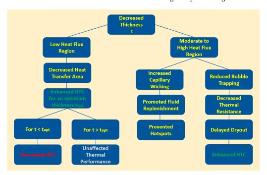
**Figure 19.** Diagram summarizing the impact of a metal foam attachment thickness on the pool boiling of a commercial coolant. Adapted from [149].
