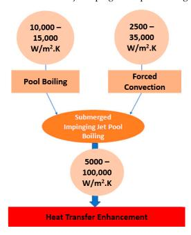
**Figure 8.** Schematic diagram showing the typical ranges of the heat transfer coefficients of the mechanisms involved in submerged impinging jet pool boiling. Adapted from [60].
