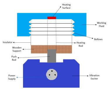
Figure 2. Schematic diagram of a surface vibration apparatus. Adapted from [33].
