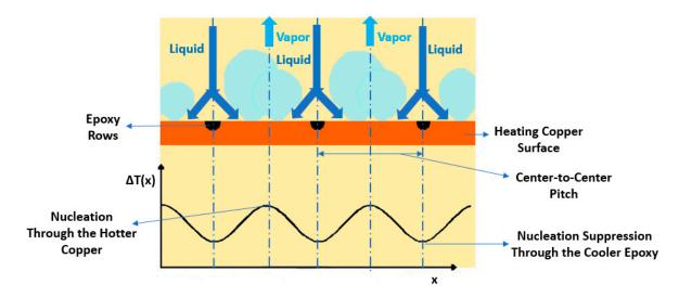
**Figure 18.** Schematic diagram and plot regarding the nucleation and liquid/vapor separation on a bi-conductive surface. Adapted from [147].
