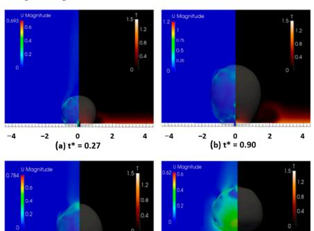
fluid. Figure 17 presents some of the results of the velocity, magnitude, and temperature during bubble growth.
