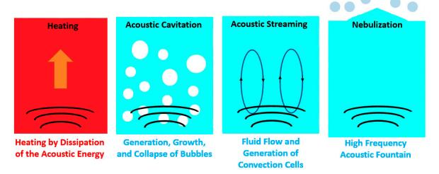
**Figure 3.** Schematic diagram representing the ultrasound-assisted pool-boiling-related phenomena. Adapted from [40].
