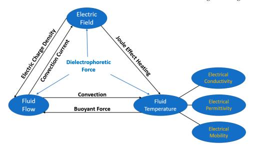
Figure 6. Schematic diagram of the electrohydrodynamic (EHD) interactions. Adapted from [51].
