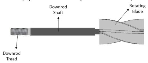
Figure 4. Scheme of a four-blade rotating blade. Adapted from [45].
