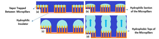
**Figure 15.** Schematic diagram of the nucleate boiling process stages using a biphilic heating surface with micropillar arrays: (a) vapor bubbles generated between the micropillars; (b) vapor bubbles merge, forming larger bubbles; (c) isolated bubbles at low superheats; (d) jets of columns at high superheats. Adapted from [133].
