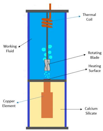
Figure 5. Schematic diagram of the set-up with a four-blade rotating blade. Adapted from [45].
