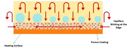
**Figure 11.** Schematic representation of the capillary wicking effect on a porous coating. Adapted from [91].
