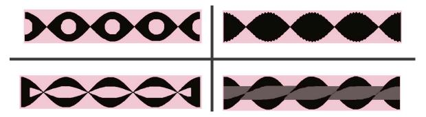
Figure 21. Typical sections of perforated and non-perforated swirl flow inserts. Adapted from [157].
