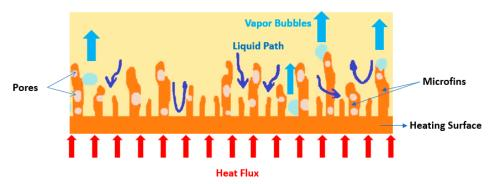
**Figure 14.** Schematic illustration of the liquid–vapor interactions on a surface with microfins and pores. Adapted from [121].
