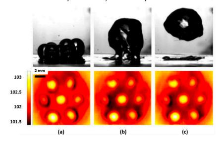
**Figure 16.** Synchronized images and thermographical images of the bubbles generated in seven hydrophobic spots with a spacing equal to the diameter of the bubbles. The (**a–c**) conditions refer to before, during, and after coalescence, respectively [75].
