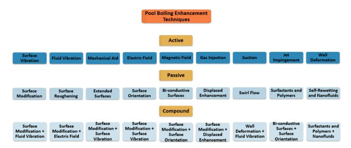
Figure 1. Main pool boiling enhancement techniques.
