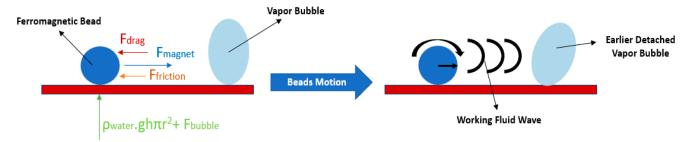
**Figure 7.** Schematic diagram of the actuating forces and principle of actuation of the beads. Adapted from [53].
