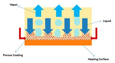
**Figure 12.** Schematic representation of the separation of the liquid and vapor paths on a porous coating. Adapted from [91].
