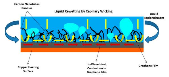
**Figure 10.** Schematic representation of the liquid replenishment process through the capillary wicking effect of CNT bundles. Adapted from [82].
